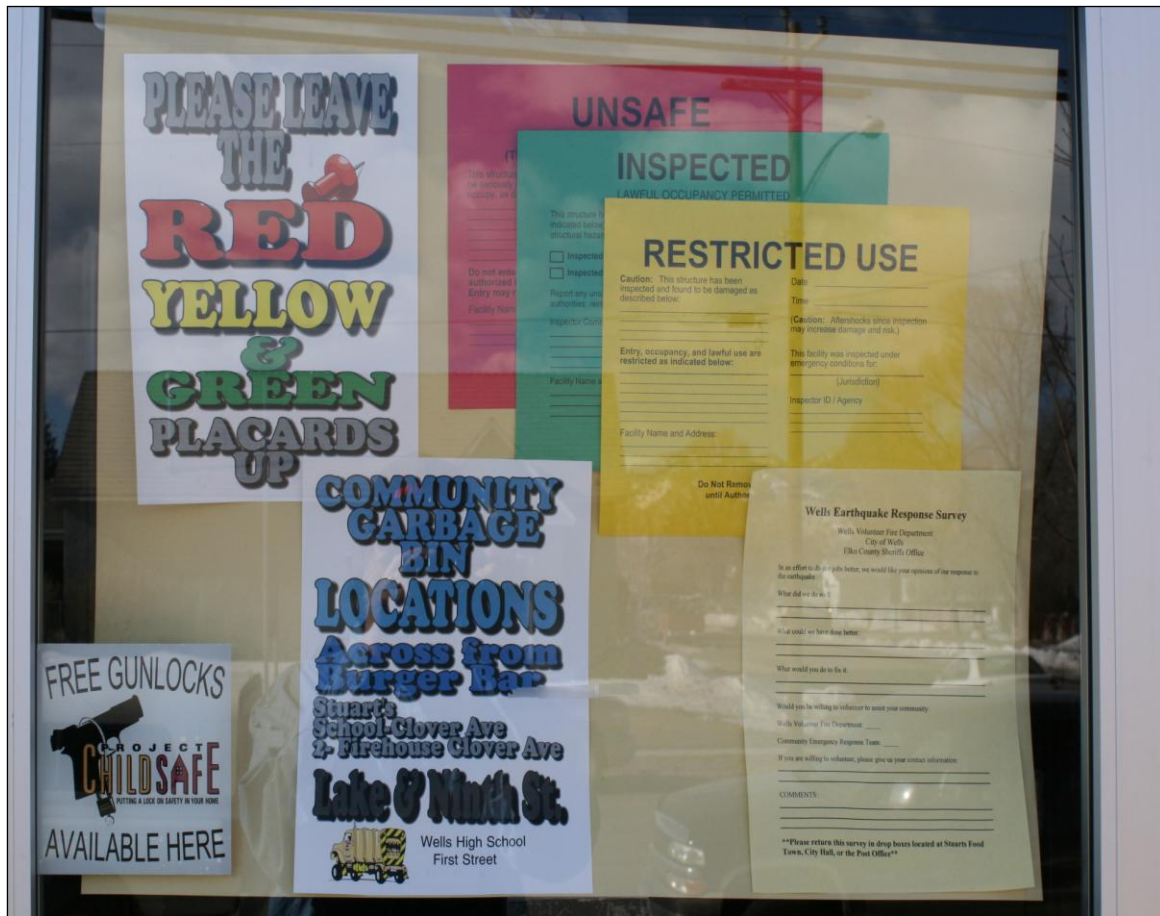
Figure 14. A public display board explains the meaning of the different colored placards used to indicate inspected houses and their post-earthquake condition.
