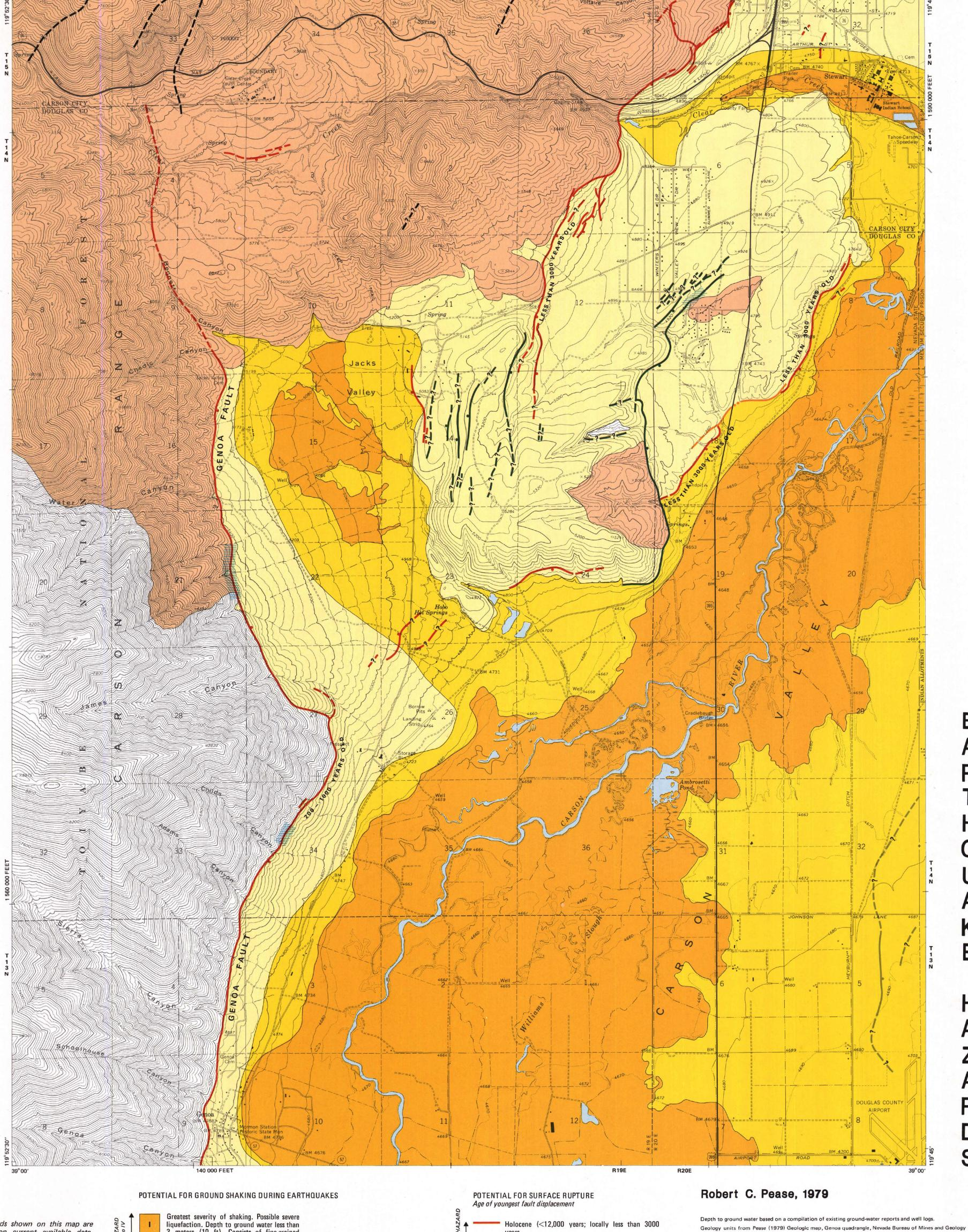
The hazards shown on this map are based upon current available data. Shaking characteristics are inferred from interpretation of geologic, seismic velocity, soils engineering, and ground-water information. Surface rupture potentials are inferred from generalized geologic and soils (weathering profile) information.
