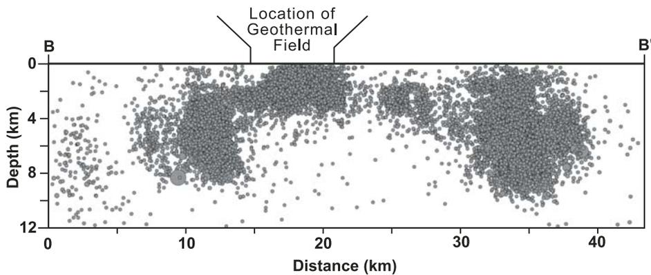
Figure 7. NE-SW cross section B-B' showing hypocenters beneath the Coso Range for more than 40,000 events ranging in magnitude from -1 to 5.2.
