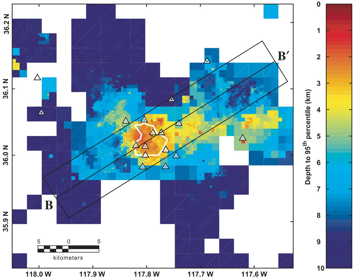
Figure 6. Maximum depth of seismicity as determined by the 95th percentile of hypocenters. Events are binned into boxes, the sizes of which are determined by event density, e.g., smaller boxes in areas of greater density. B–B' is shown in Figure 7.
