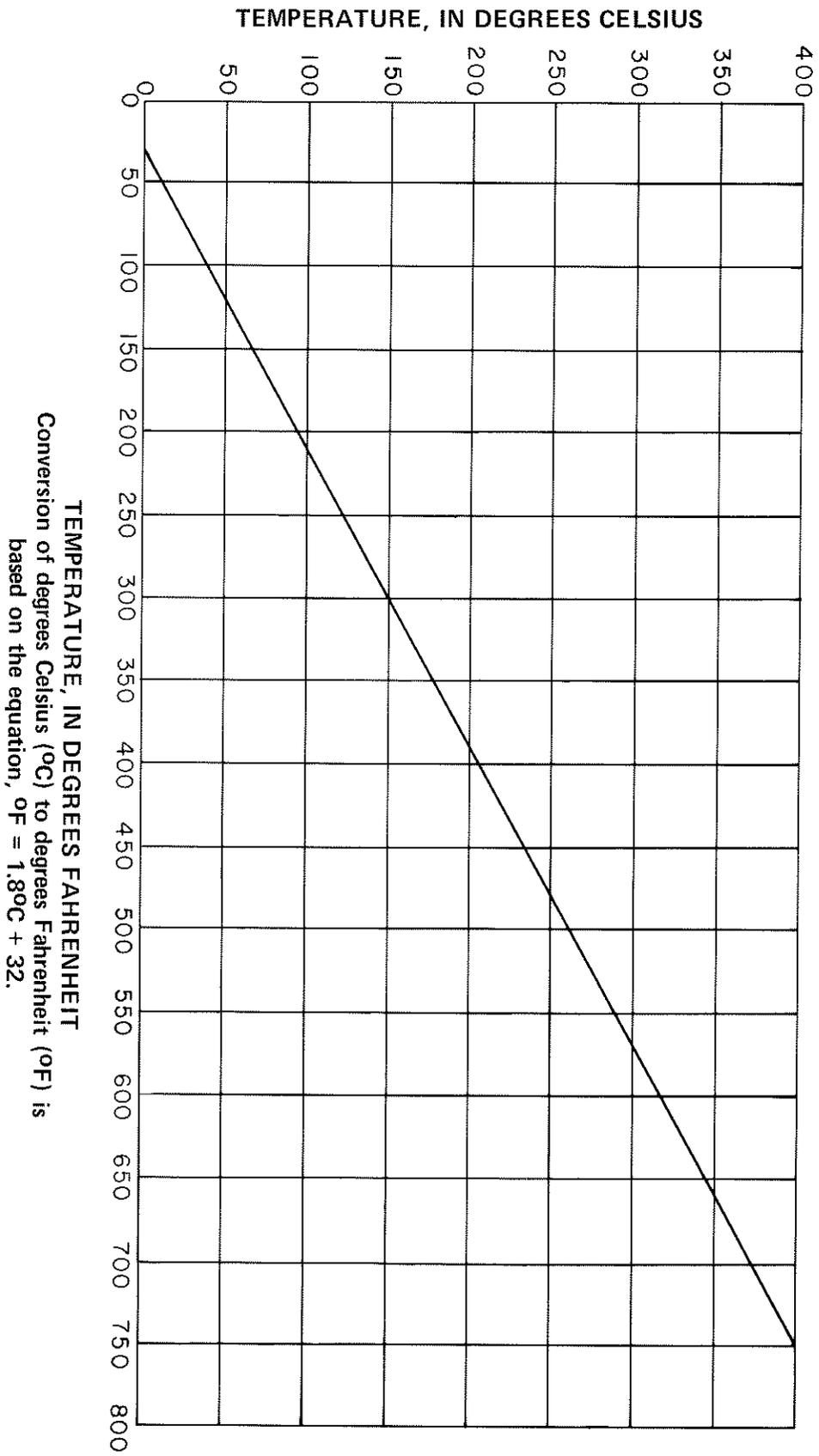
FIGURE 3. Temperature-conversion graph.
