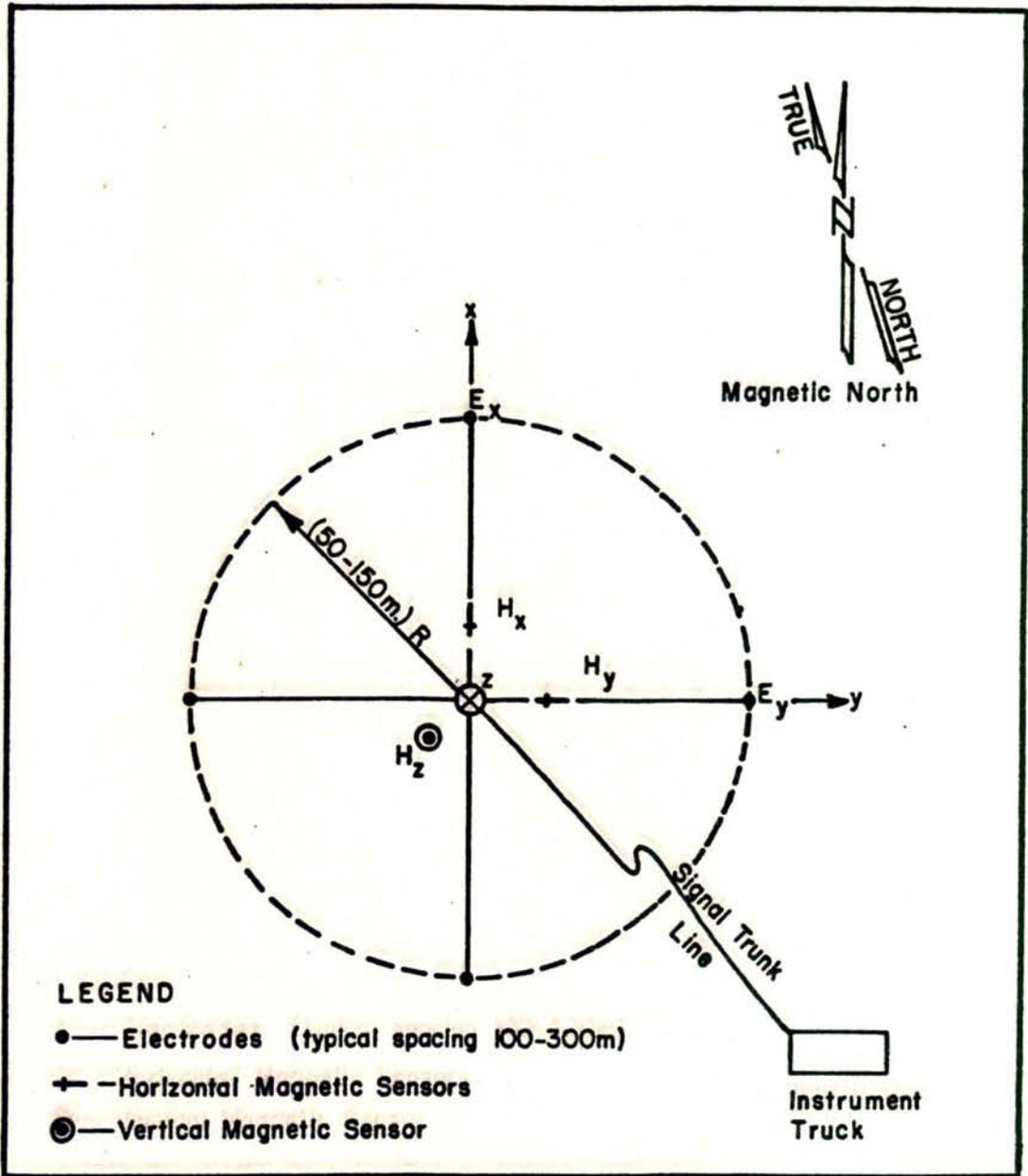
Fig. A-1: Magnetotelluric Field Sensor Layout.
