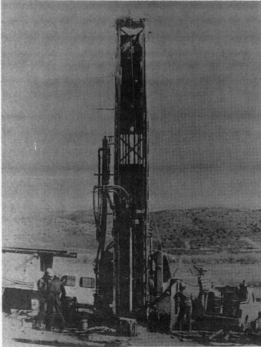
Figure A 2 . Photograph of Schramm Rotadrill CF 15 drill rig.
