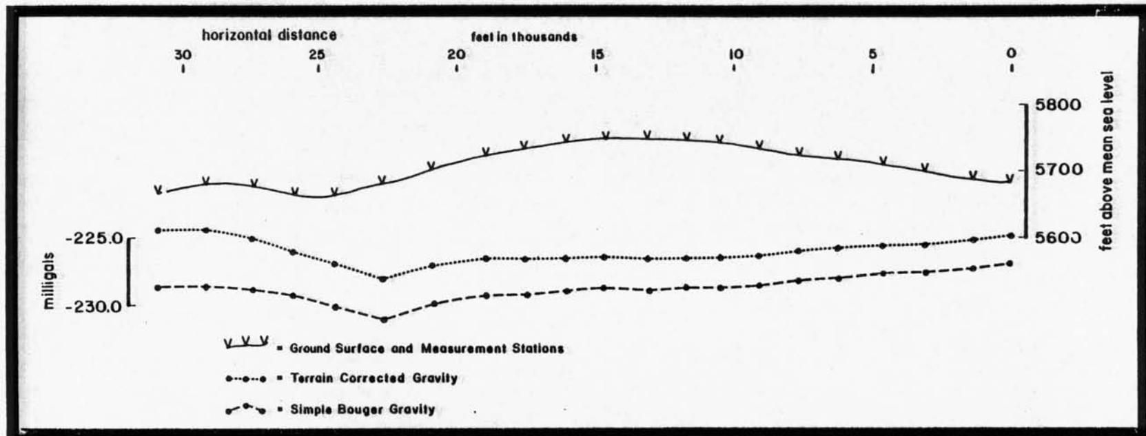
Figure C9. Simple and complete Bouguer anomaly, and topography of gravity traverse BA.
