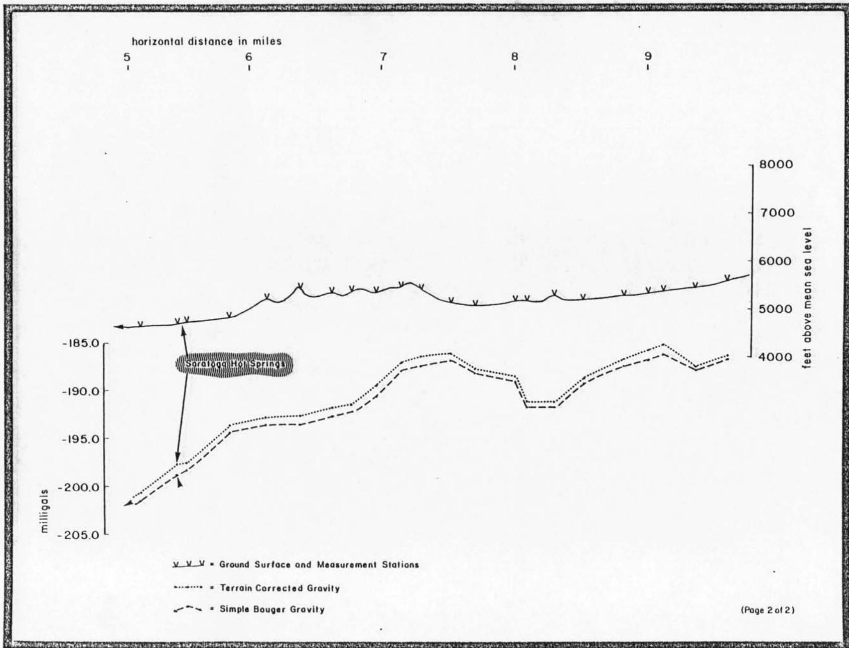
Figure B8b . HS gravity traverse, eastern section.
