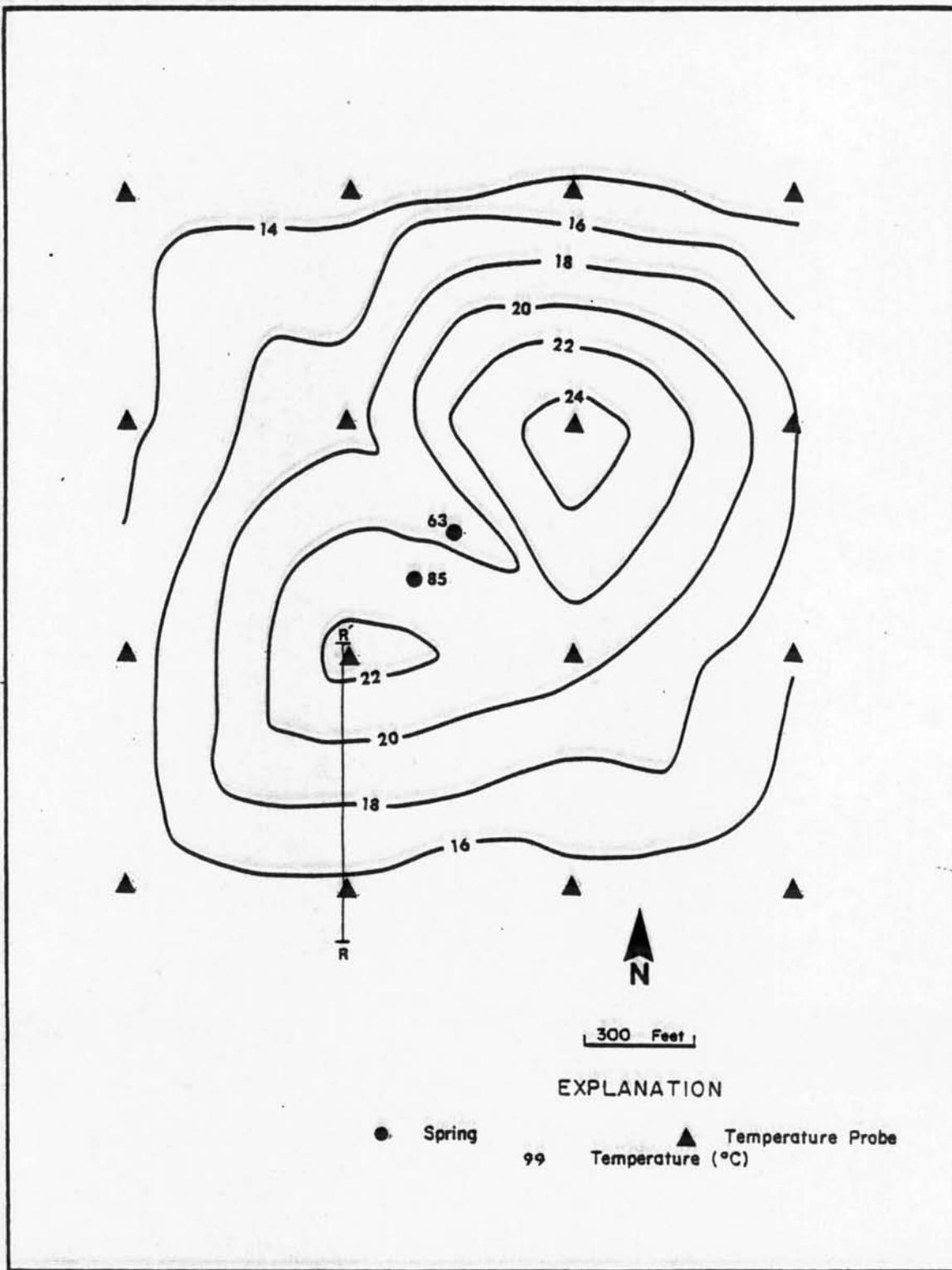
Figure C 25. Two meter probe isotherm configuration at McLeod Ranch Hot Springs. Line R-R' represents the path used during shallow resistivity study (see text under shallow resistivity heading for discussion).
