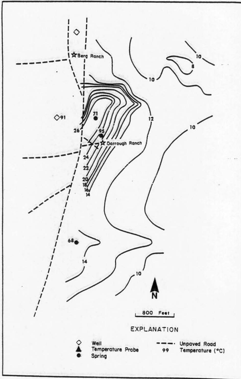
Figure C 26. Two meter probe isotherm configuration at Darrough's Hot Springs. Scale of the figure prohibits probe locations from being depicted.
