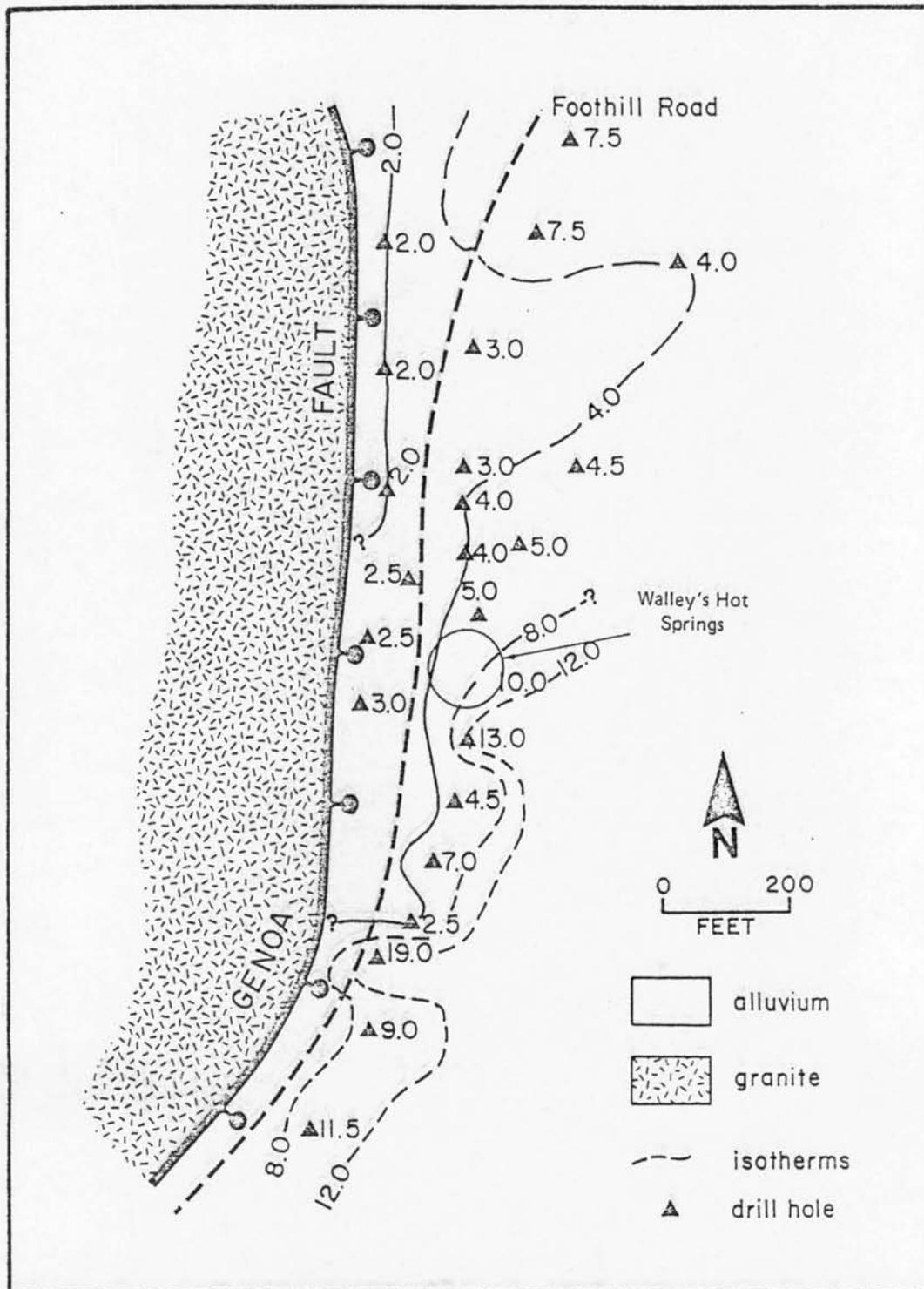
Figure B23. Spatial relationship between shallow temperature gradients and nearby mapped faults. See text for explanation. Ball on downthrown side of fault. (after Gar-side and Schilling, 1979)
