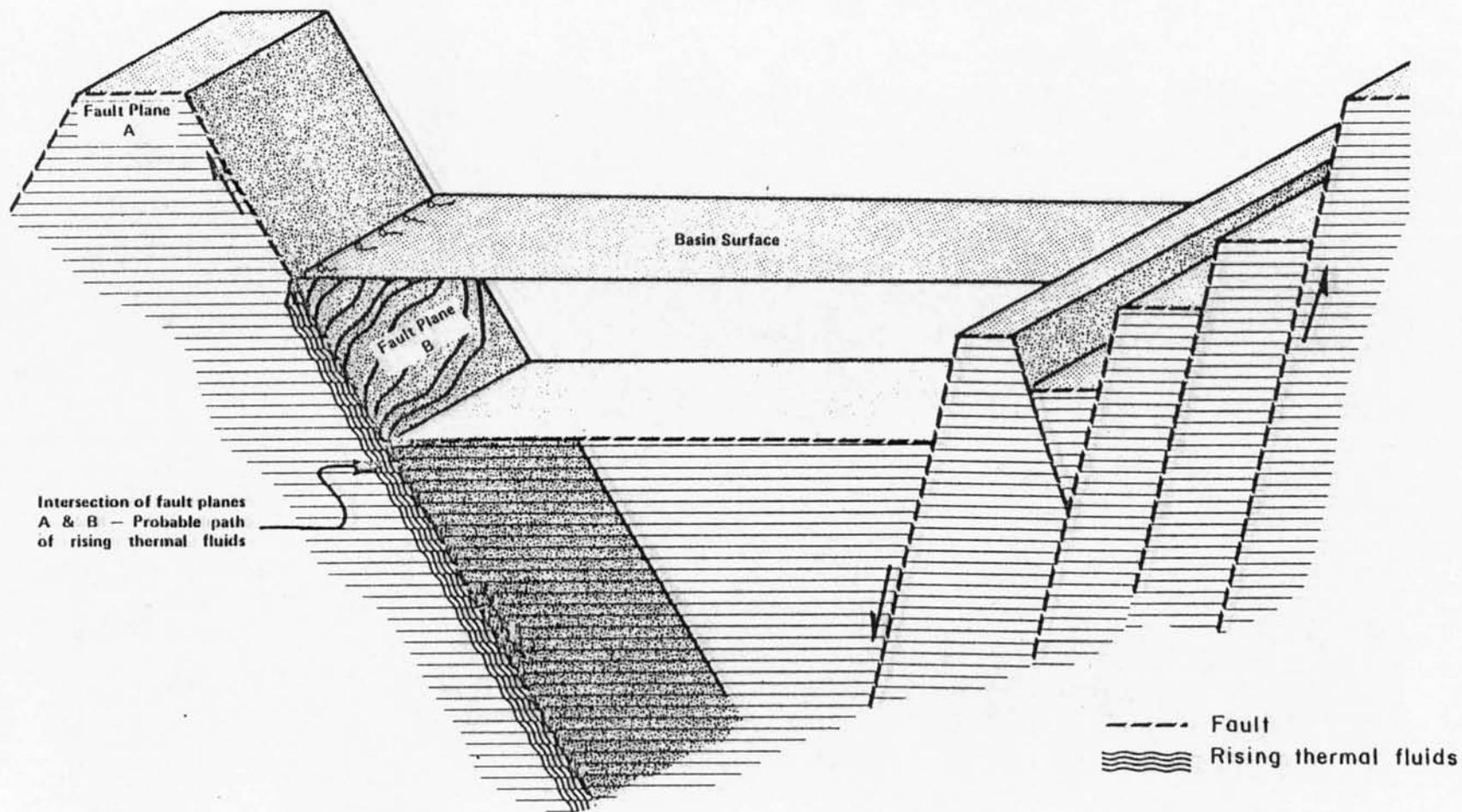
Figure B32. Graphic model showing the inferred structural controls on the upwards migration of geothermal fluids in the Carson-Eagle Valley study area.
