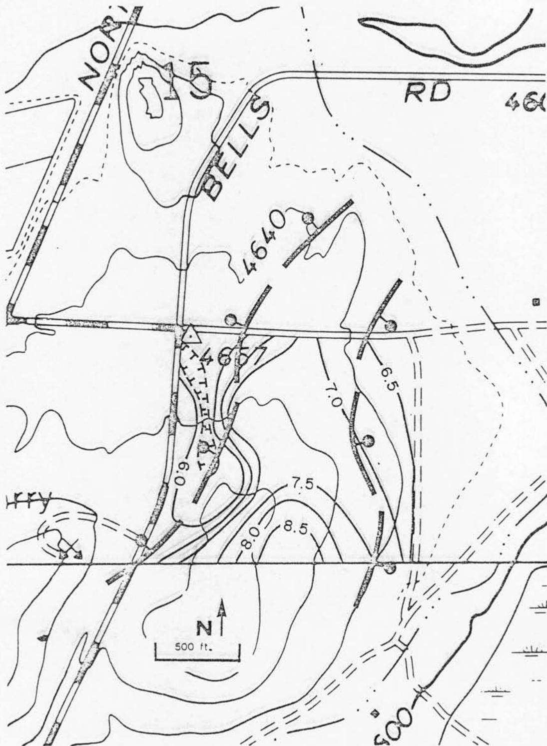
Figure B22. Shallow depth isotherms and mapped faults at drill site CC-1. Ball on down-thrown side of fault. (after Binger, 1978)
