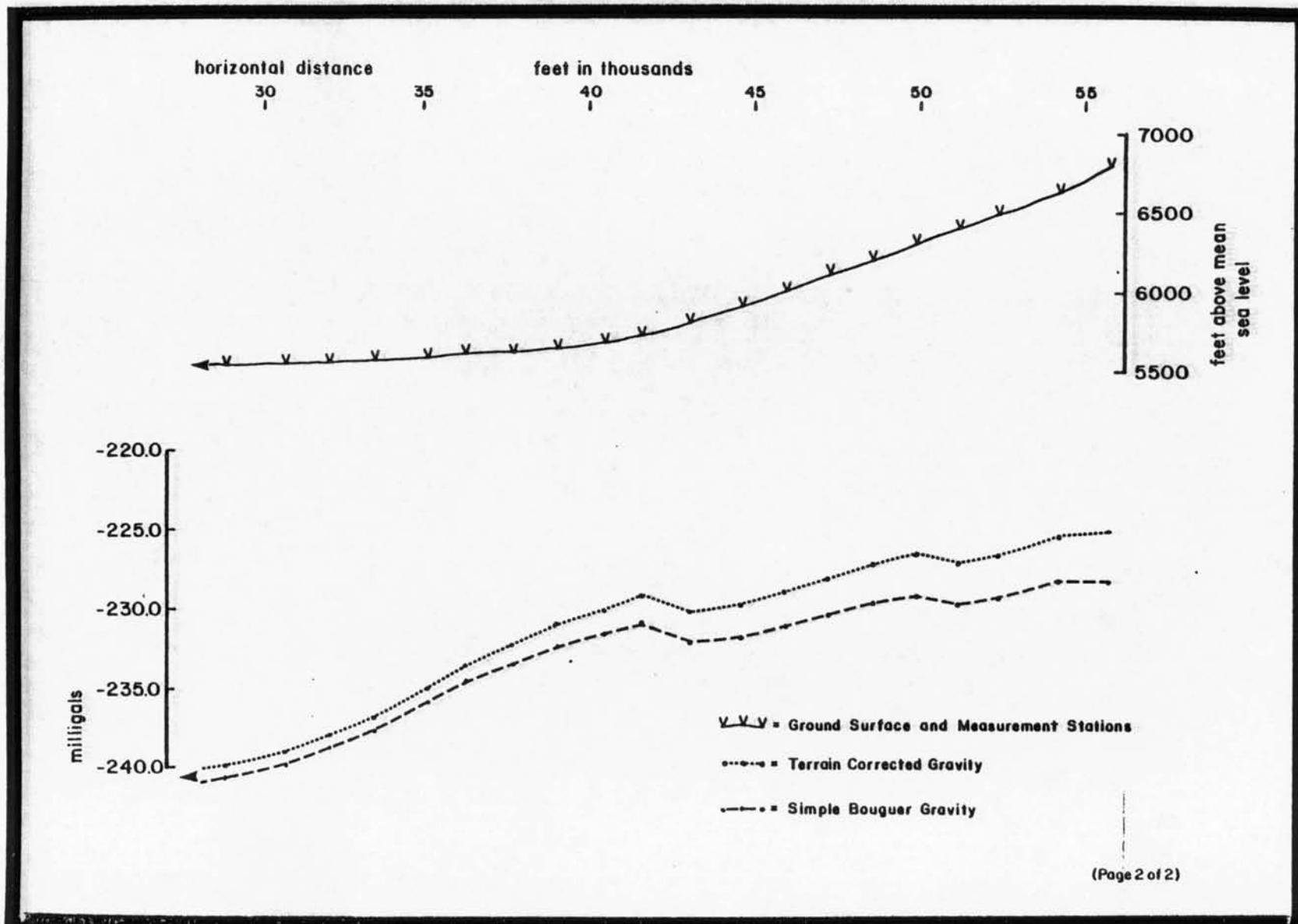
Figure C8b. Simple and complete Bouguer anomaly, and topography of the eastern segment of the D (Darrough) gravity traverse.
