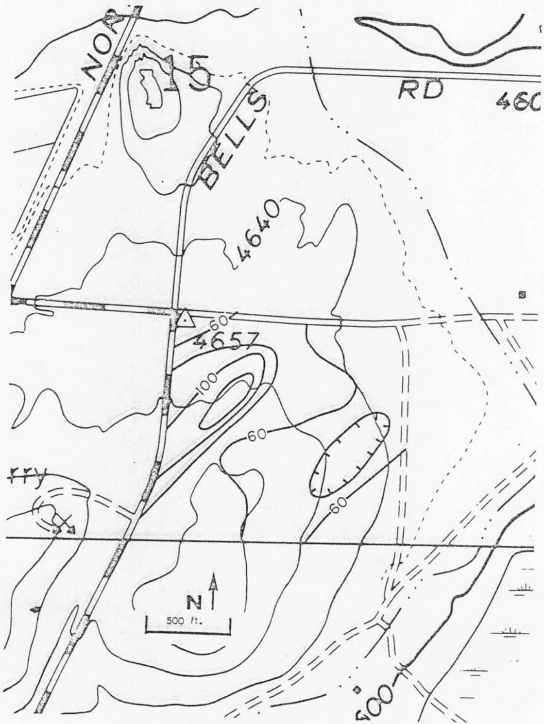
Figure B26. Contour map of mercury (concentrations in ppb) in soil sample at drill site CC-1.
