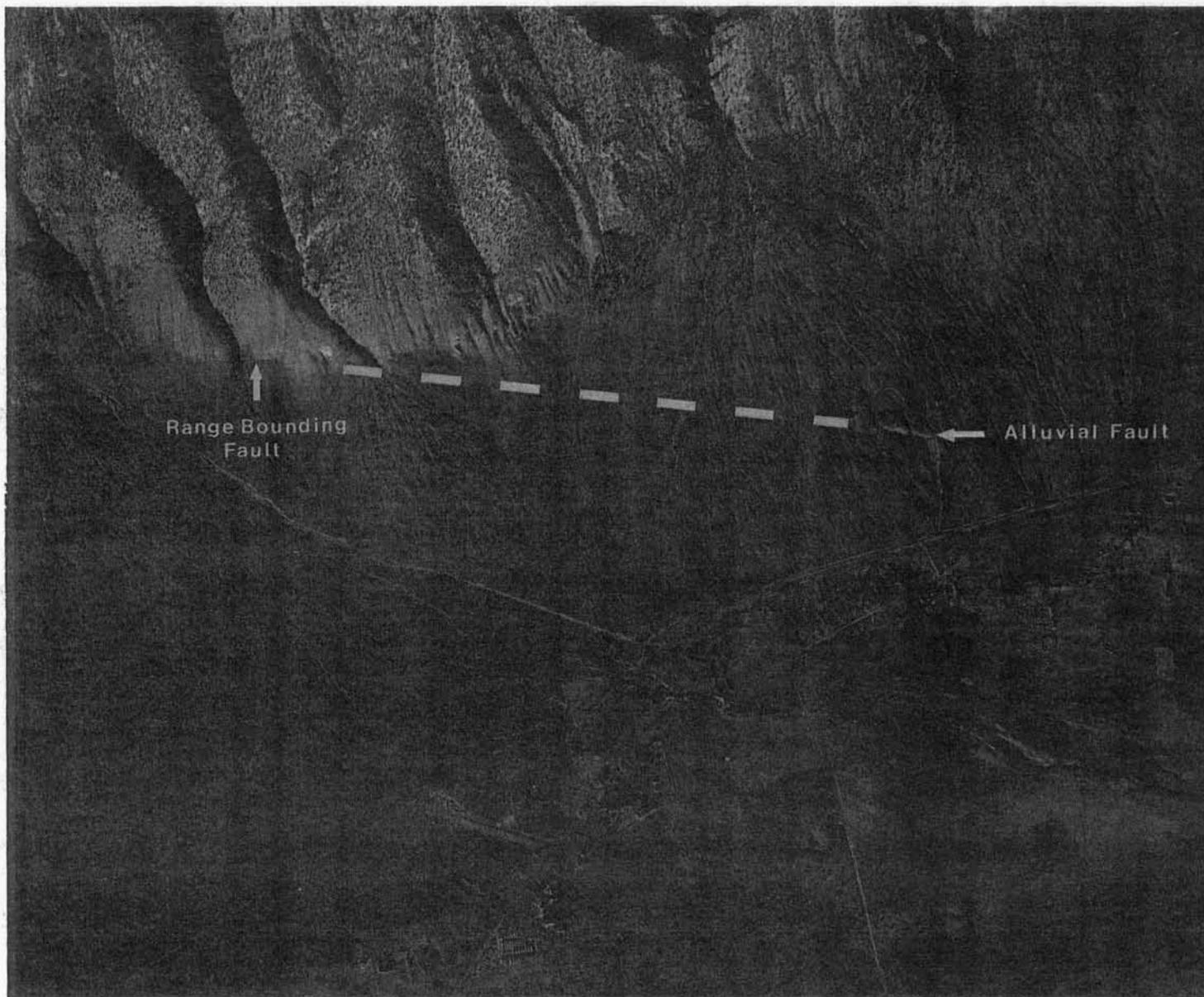
Figure C16 . Low sun-angle photography of range bounding and alluvial fault traces southwest of Darrough's Hot Springs, scale 1:24,000. Note colinear trend as shown by dashed line.
