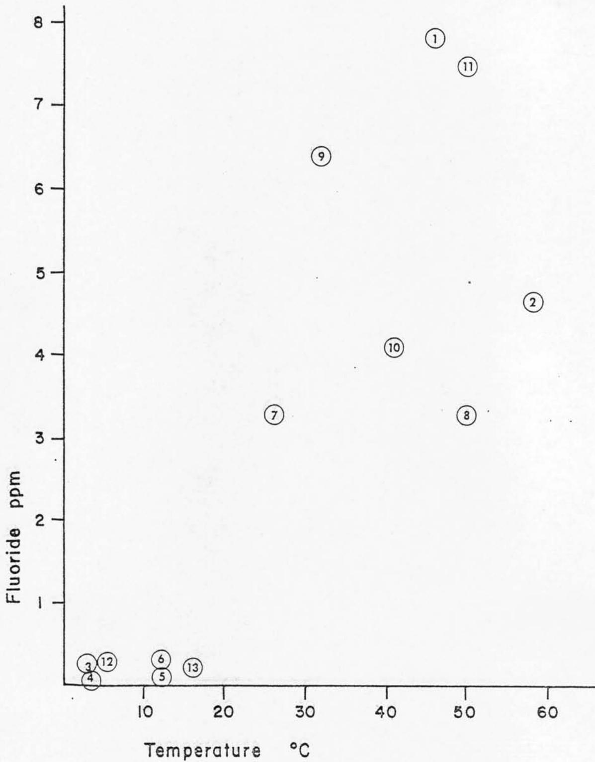
Figure B19. Relationship between temperature and fluoride concentrations for waters from Carson-Eagle Valley study area. Circled numbers refer to CW sample numbers in Table B1.
