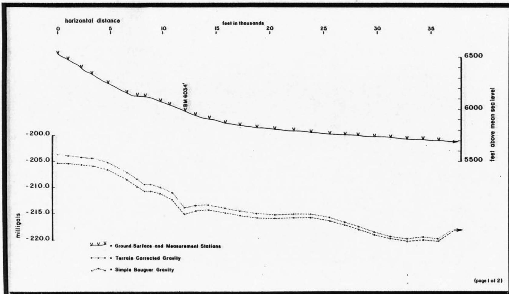
Figure C5a . Simple and complete Bouguer anomaly, and topography of the western segment of the S (Spencer's) gravity traverse.
