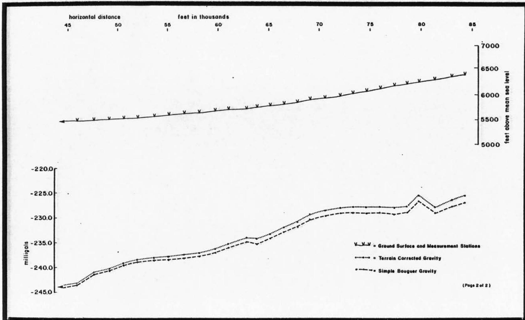
Figure C6b . Simple and complete Bouguer anomaly, and topography of the eastern segment of the MR (McLeod Ranch) gravity traverse.
