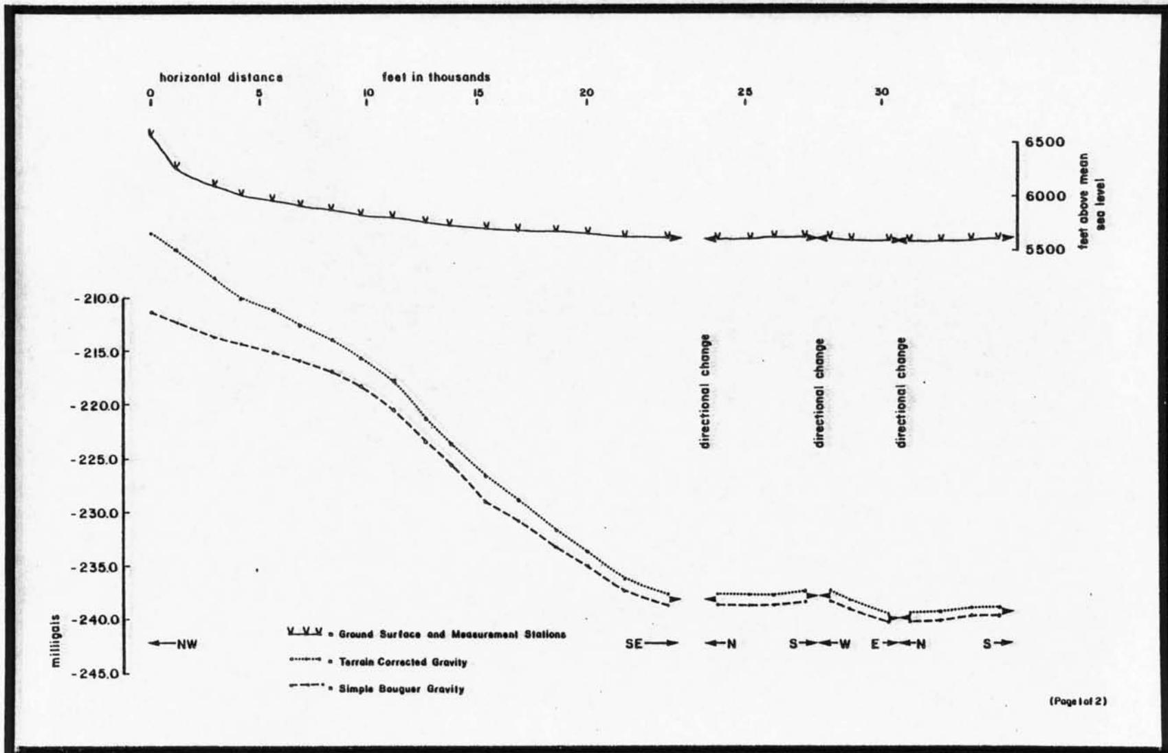
Figure C7a. Simple and complete Bouguer anomaly, and topography of the western segment of the OMC (Ophir-Moore's Creek) gravity traverse.
