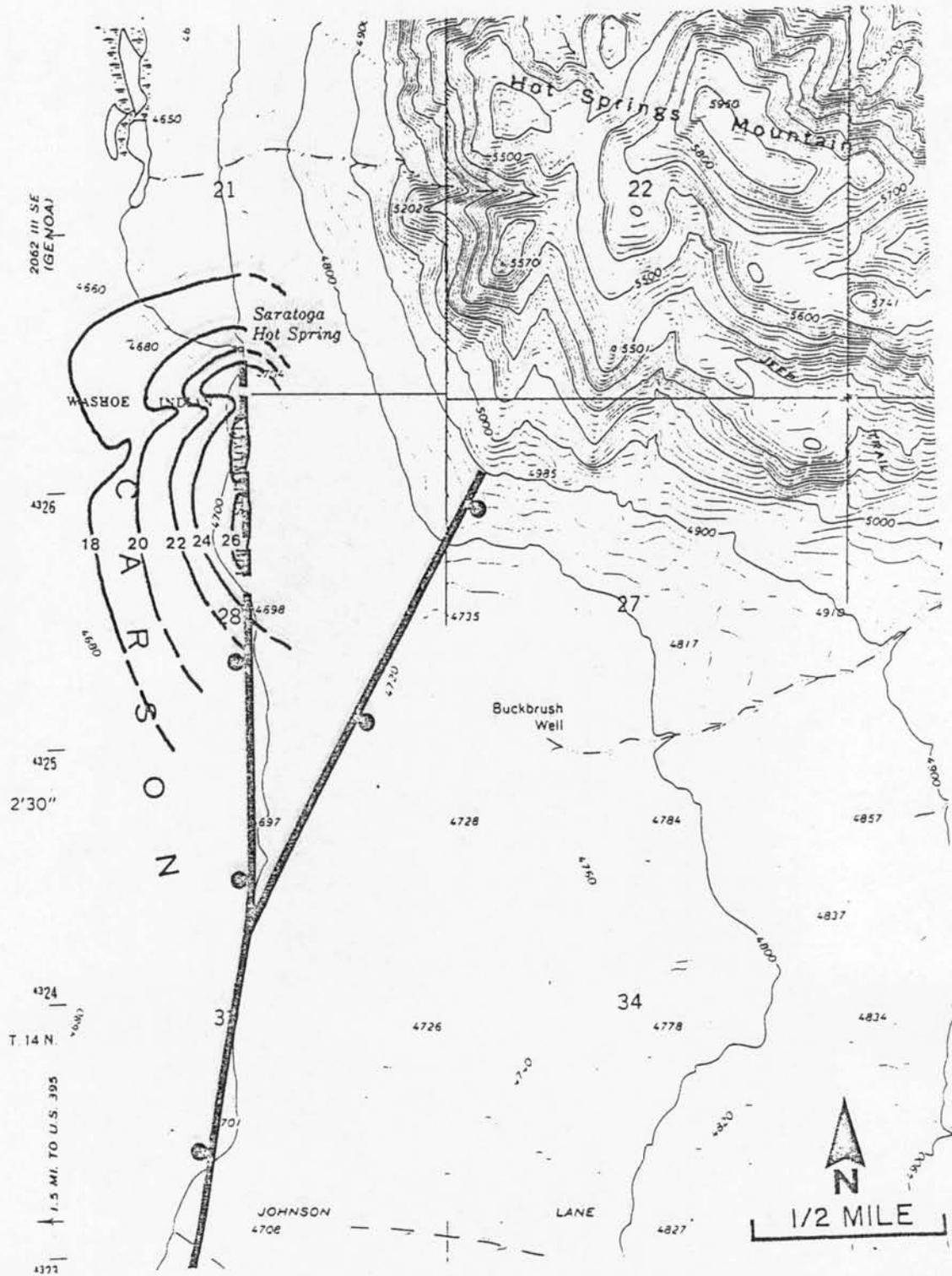
Figure B21. Spatial relationship between Saratoga 2 m. temperature probe isotherms and nearby fault (modified after Moore, 1979). Isotherm contour interval is 2°C; ball on downthrown side of fault.
