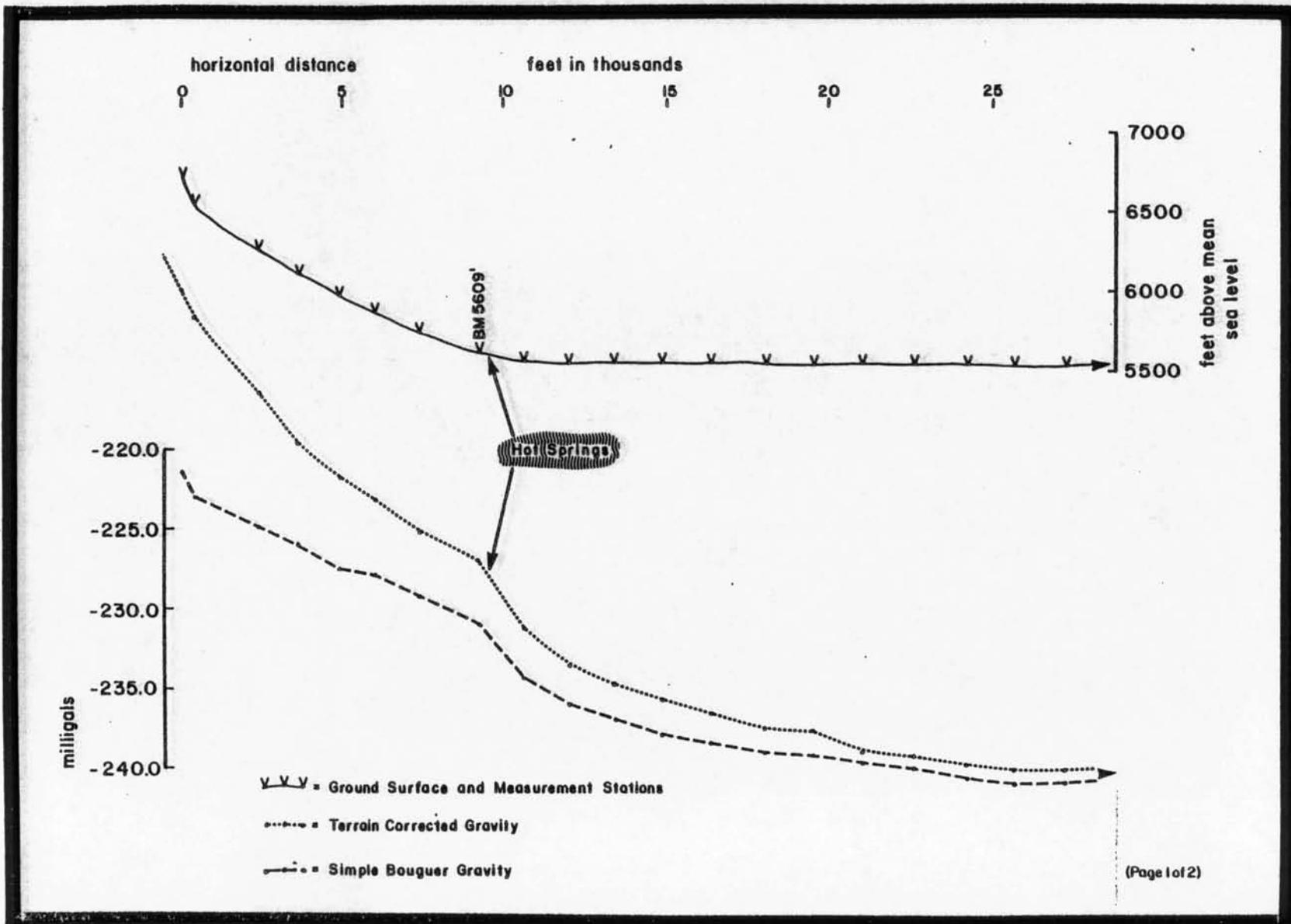
Figure C8a . Simple and complete Bouguer anomaly, and topography of the western segment of the D (Darrough) gravity traverse.
