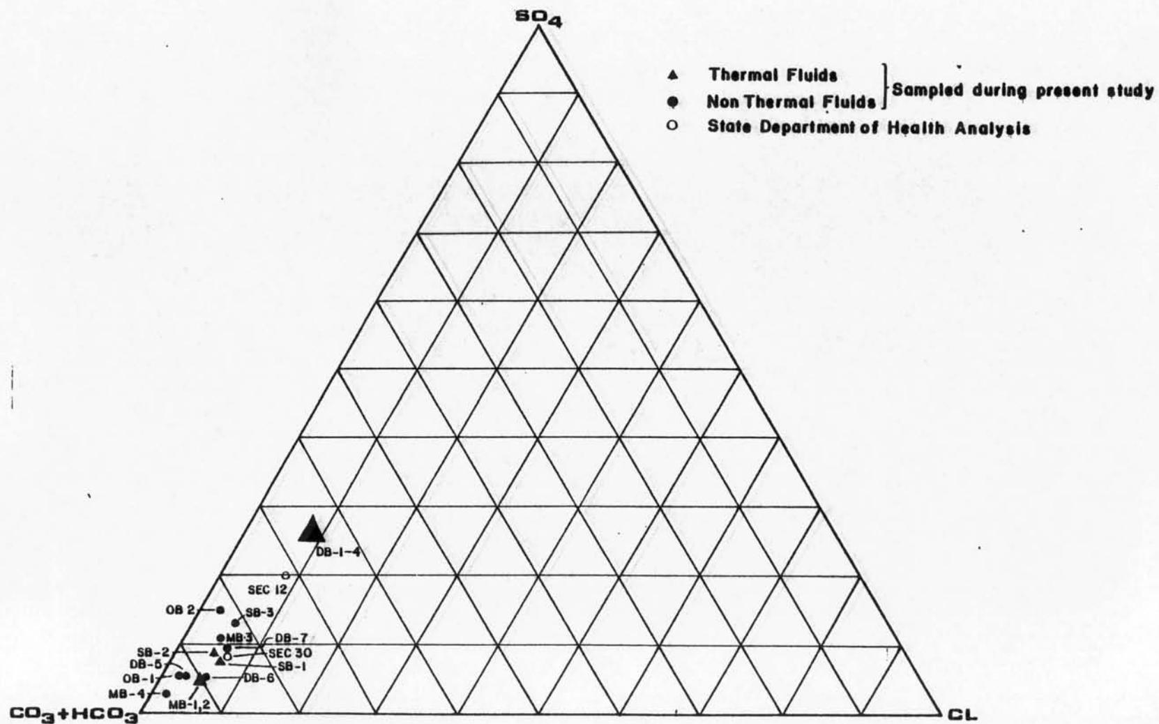
Figure C 21. Distribution of thermal and non-thermal fluids with respect to  $\text{CO}_3 + \text{HCO}_3 - \text{SO}_4 - \text{Cl}$  anions in the Big Smoky Valley. Points are plotted as percent equivalents per million of the sum for the species.
