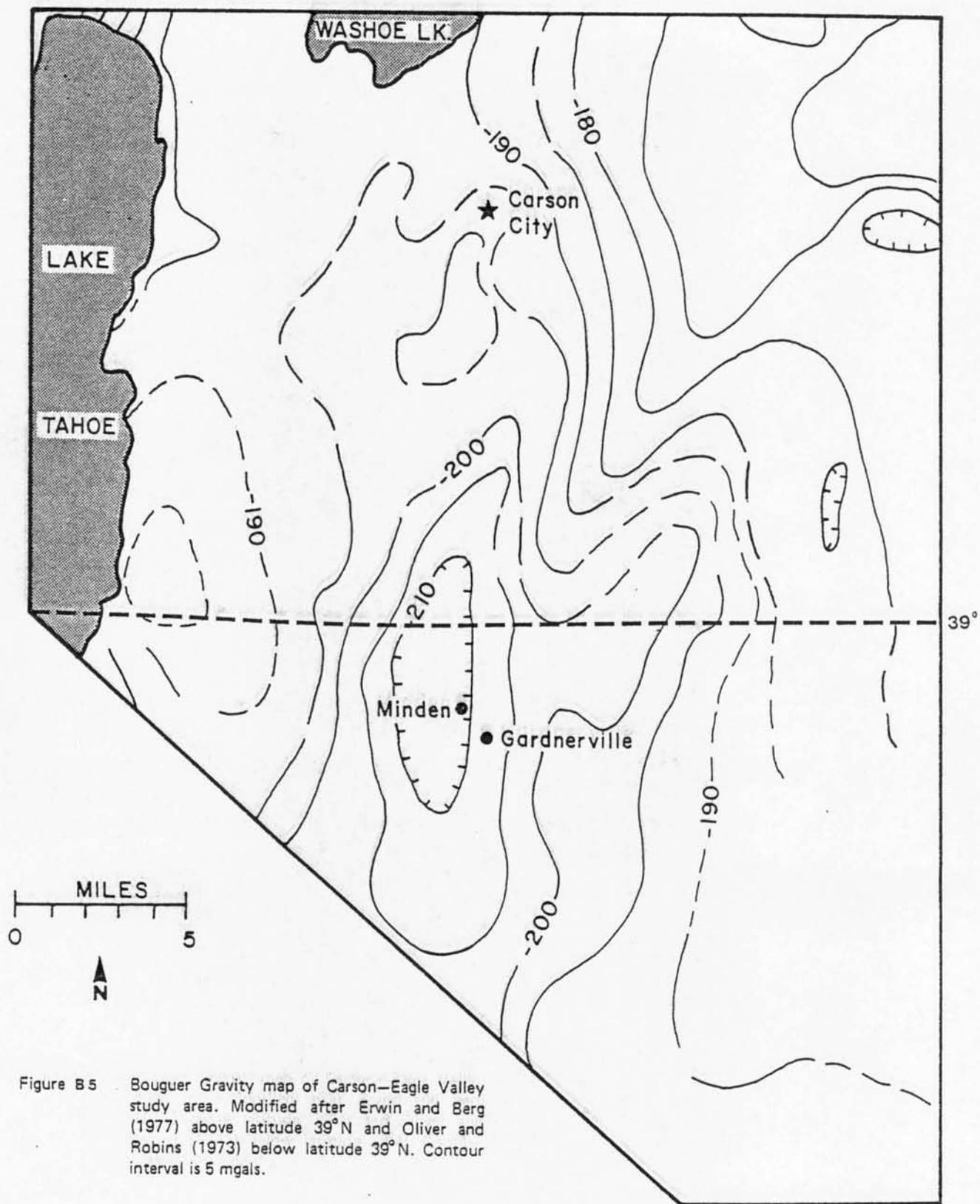
Figure B5 Bouguer Gravity map of Carson-Eagle Valley study area. Modified after Erwin and Berg (1977) above latitude 39°N and Oliver and Robins (1973) below latitude 39°N. Contour interval is 5 mgals.
