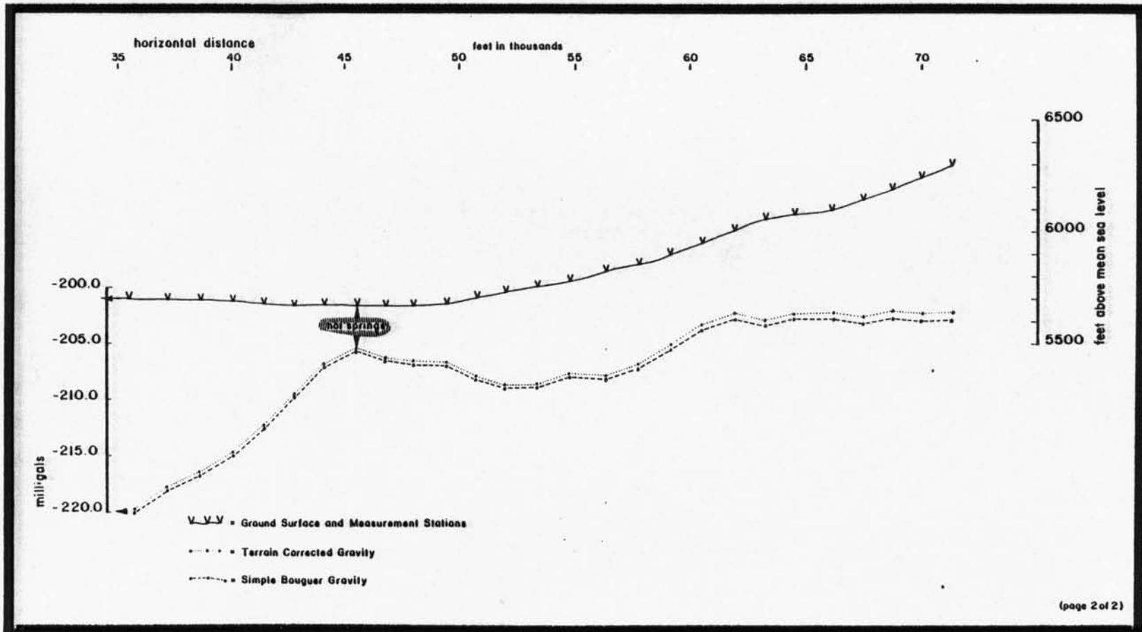
Figure C5b. Simple and complete Bouguer anomaly, and topography of eastern segment of the S (Spencer's) gravity traverse.
