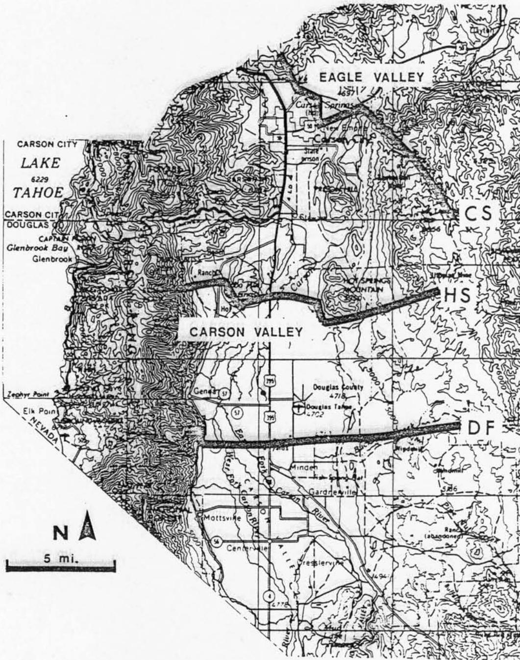
Figure B6. Location of gravity traverses CS, HS and DF in the Carson-Eagle Valley Area.
