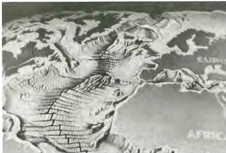
Bathymetric view of the Atlantic Ocean and the tectonically active mid-Atlantic Ridge. The ridge is a slow spreading center that is pushing the Eurasian and North American plates apart at a rate of 2.8 to 5 centimeters per year. Sediments fan out on the ocean basin, burying the basement rock in deposits up to 14 kilometers thick. Photo courtesy of Celestial Arts.
