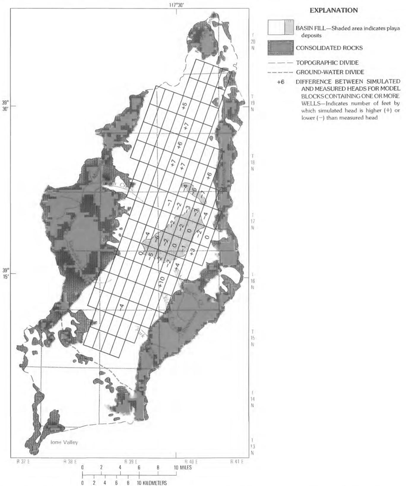
FIGURE 16.—Difference between simulated and measured (averaged over 2 mi<sup>2</sup> model blocks) heads in model layer one for the steady-state solution.
