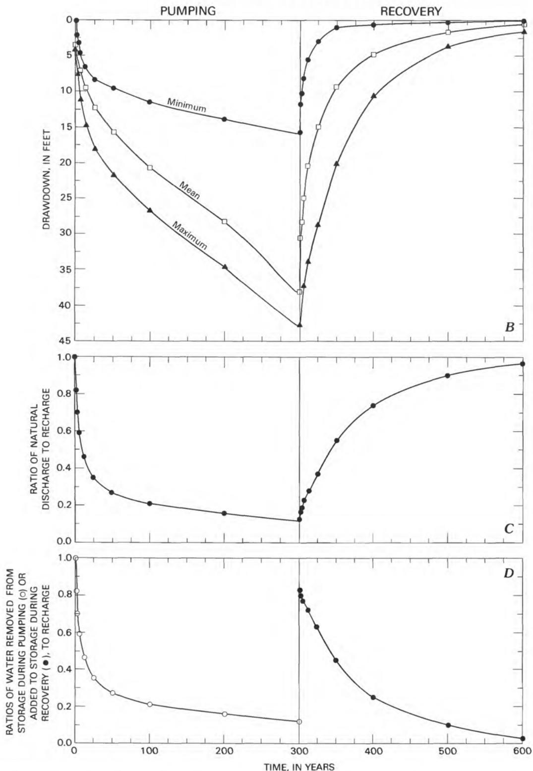
FIGURE 21—Continued.—Results of simulated pumping and subsequent recovery for scenario B. *B*, Water-level declines during pumping, and subsequent water-level recoveries; shows maximum, mean, and minimum drawdowns for the model blocks containing pumped wells. *C*, Changes in the ratio of natural discharge to recharge during pumping and recovery. *D*, Changes in the ratios of (1) water removed from storage during pumping to recharge and (2) water added to storage during recovery to recharge.
