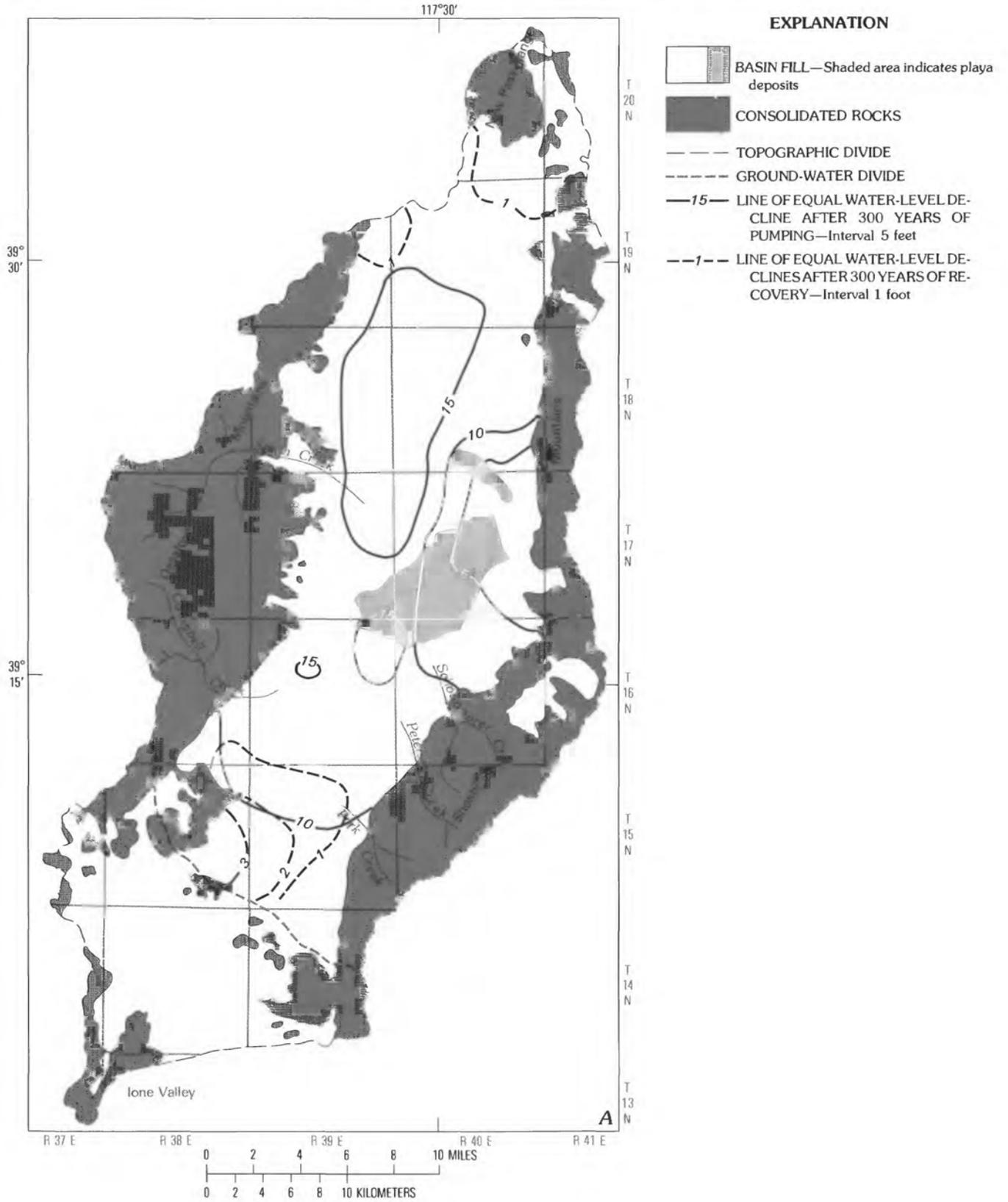
FIGURE 20 (above and facing page).—Results of simulated pumping and subsequent recovery for scenario A. Wells are distributed to most effectively reduce natural discharge, and are pumped at a combined rate equal to the sustained yield. A, Areal distribution of drawdown after 300 yr of pumping and after 300 yr of recovery.
