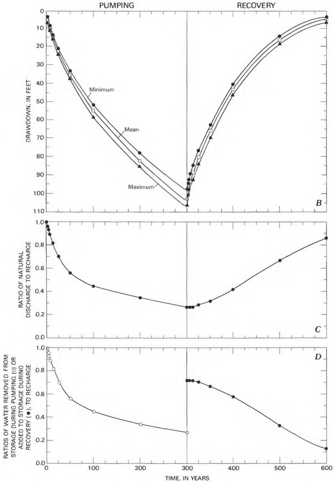
FIGURE 22—Continued.—Results of simulated pumping and subsequent recovery for scenario C. *B*, Water-level declines during pumping, and subsequent water-level recoveries; shows maximum, mean, and minimum drawdowns for the model blocks containing pumped wells. *C*, Changes in the ratio of natural discharge to recharge during pumping and recovery. *D*, Changes in the ratios of (1) water removed from storage during pumping to recharge and (2) water added to storage during recovery to recharge.
