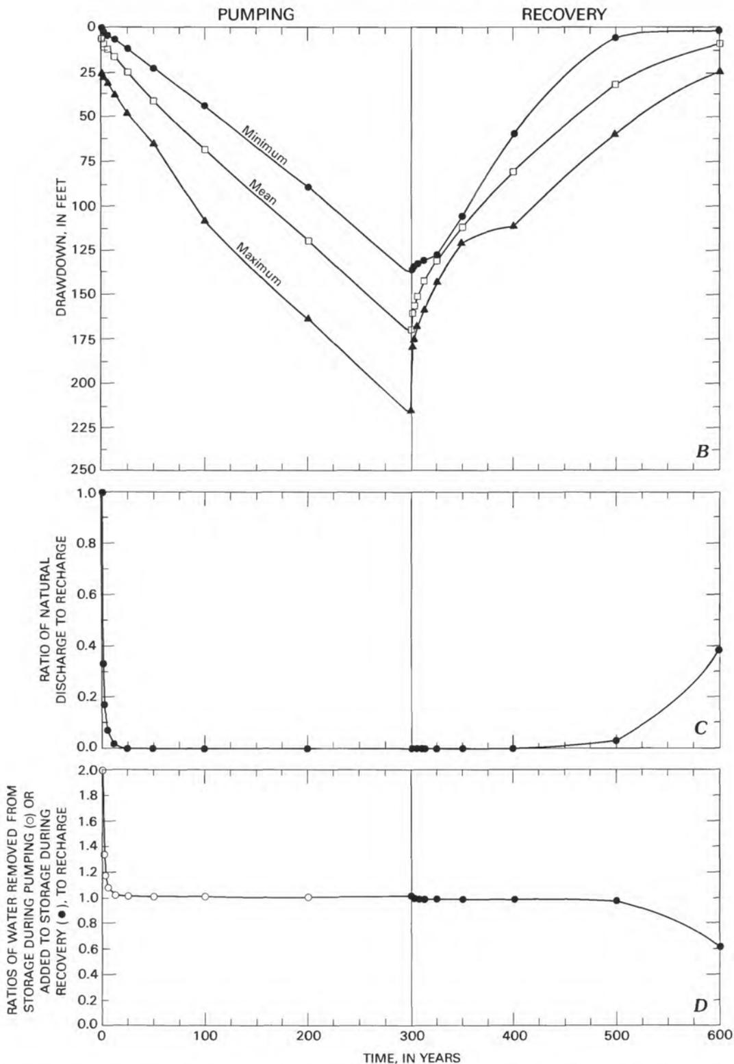
FIGURE 24—Continued.—Results of simulated pumping and subsequent recovery for scenario E. *B*, Water-level declines during pumping, and subsequent water-level recoveries; shows maximum, mean, and minimum drawdowns for the model blocks containing pumped wells. *C*, Changes in the ratio of natural discharge to recharge during pumping and recovery. *D*, Changes in the ratios of (1) water removed from storage during pumping to recharge and (2) water added to storage during recovery to recharge.
