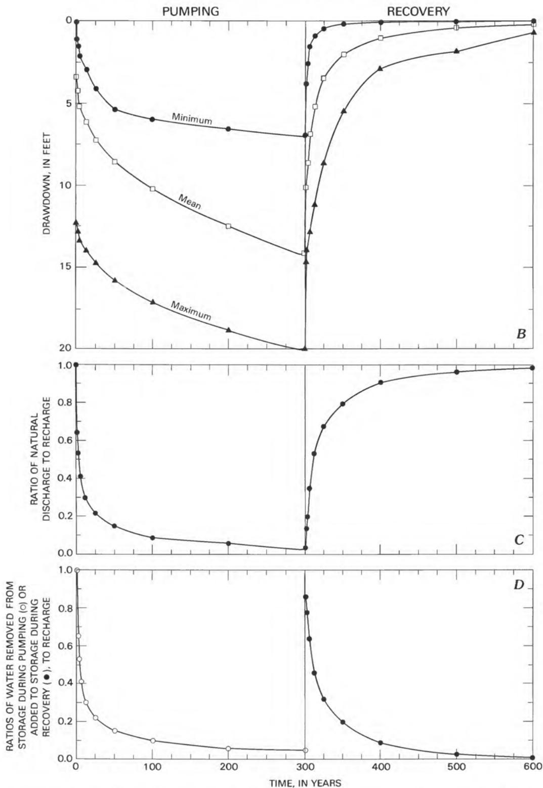
FIGURE 20—Continued.—Results of simulated pumping and subsequent recovery for scenario A. *B*, Water-level declines during pumping, and subsequent water-level recoveries; shows maximum, mean, and minimum drawdowns for the model blocks containing pumped wells. *C*, Changes in the ratio of natural discharge to recharge during pumping and recovery. *D*, Changes in the ratios of (1) water removed from storage during pumping to recharge and (2) water added to storage during recovery to recharge.
