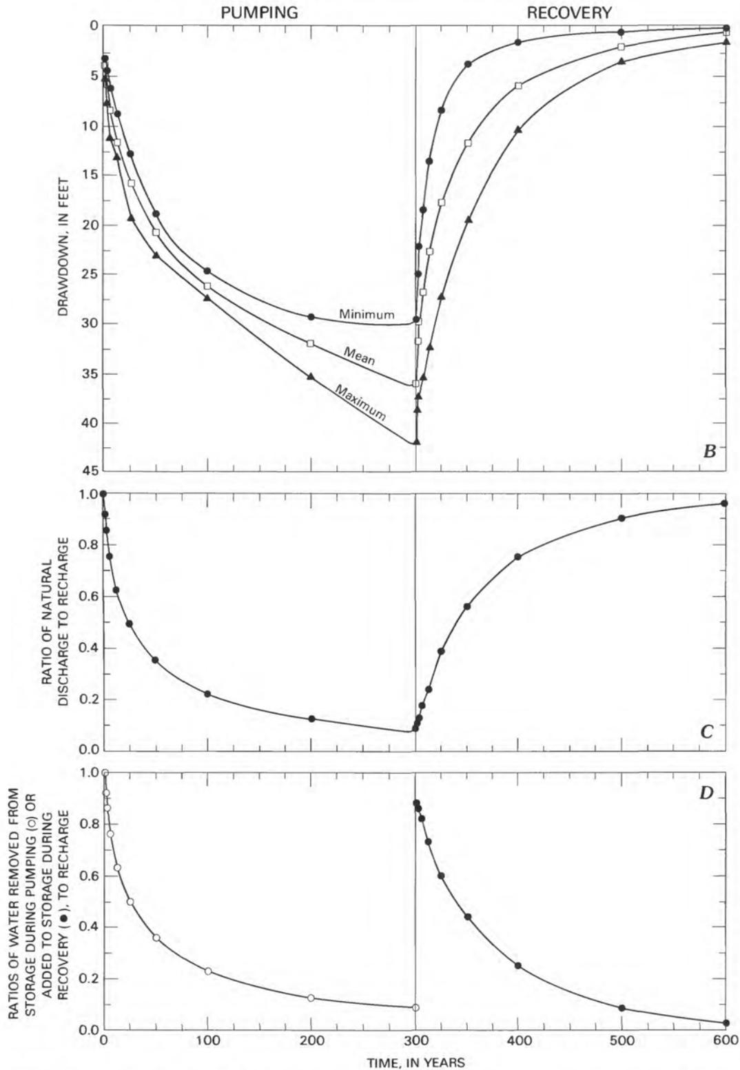
FIGURE 23—Continued.—Results of simulated pumping and subsequent recovery for scenario D. *B*, Water-level declines during pumping, and subsequent water-level recoveries; shows maximum, mean, and minimum drawdowns for the model blocks containing pumped wells. *C*, Changes in the ratio of natural discharge to recharge during pumping and recovery. *D*, Changes in the ratios of (1) water removed from storage during pumping to recharge and (2) water added to storage during recovery to recharge.
