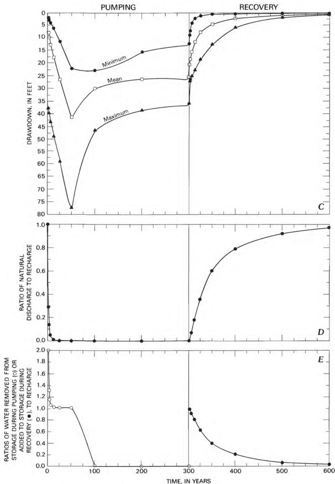
FIGURE 25—Continued.—Results of simulated pumping and subsequent recovery for scenario F. *C*, Water-level declines during pumping, and subsequent water-level recoveries; shows maximum, mean, and minimum drawdowns for the model blocks containing pumped wells. *D*, Changes in the ratio of natural discharge to recharge during pumping and recovery. *E*, Changes in the ratios of (1) water removed from storage during pumping to recharge and (2) water added to storage during recovery to recharge.
