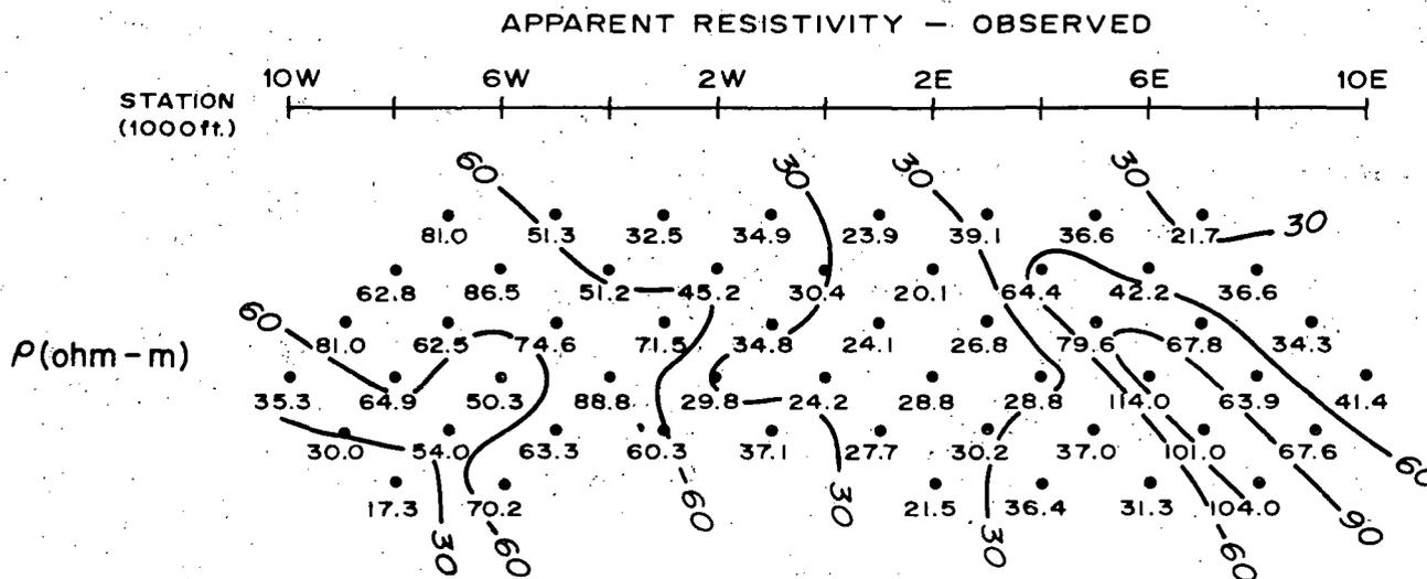
FIGURE 8 INTERPRETED RESISTIVITY SECTION AND OBSERVED APPARENT RESISTIVITY
