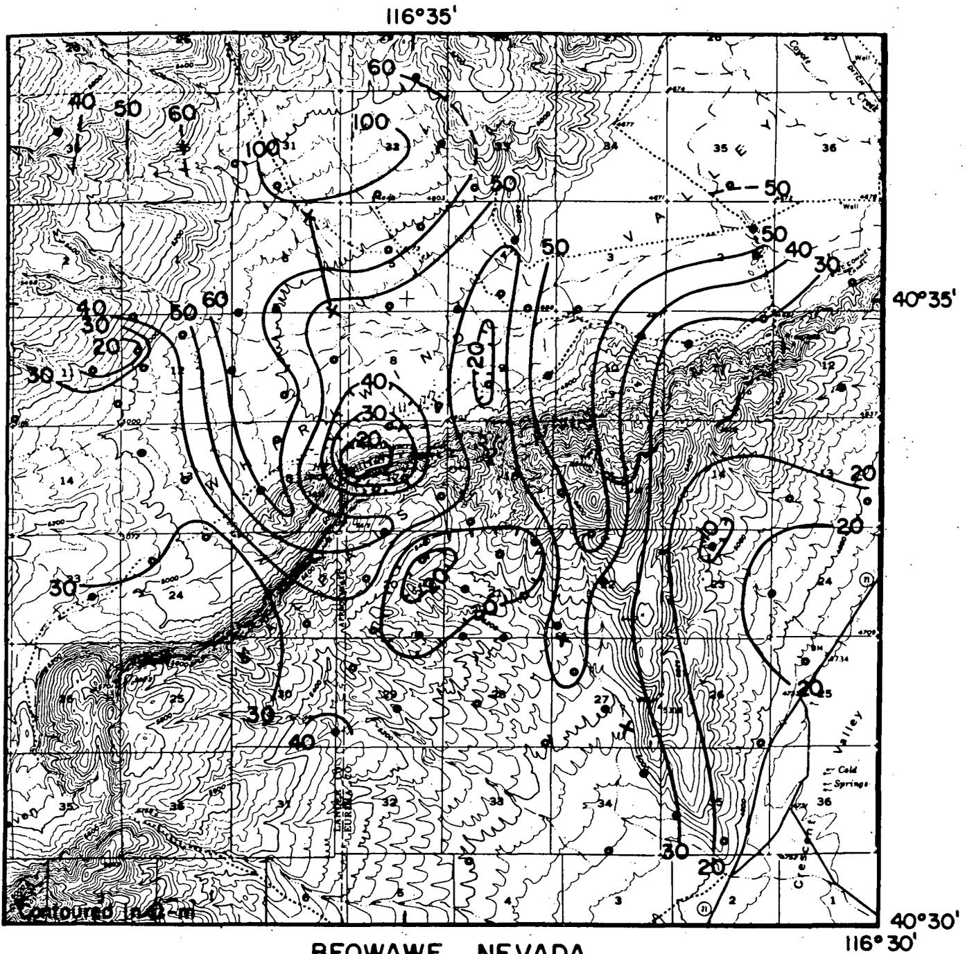
FIGURE 3 BIPOLE-DIPOLE APPARENT RESISTIVITY MAP, WHIRLWIND VALLEY TRANSMITTER (FROM WOLLENBERG AND OTHERS, 1975, LAWRENCE BERKELEY LABORATORY)
