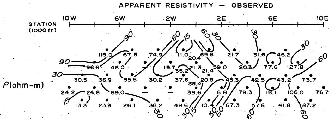
FIGURE 7 INTERPRETED RESISTIVITY SECTION AND OBSERVED APPARENT RESISTIVITY
