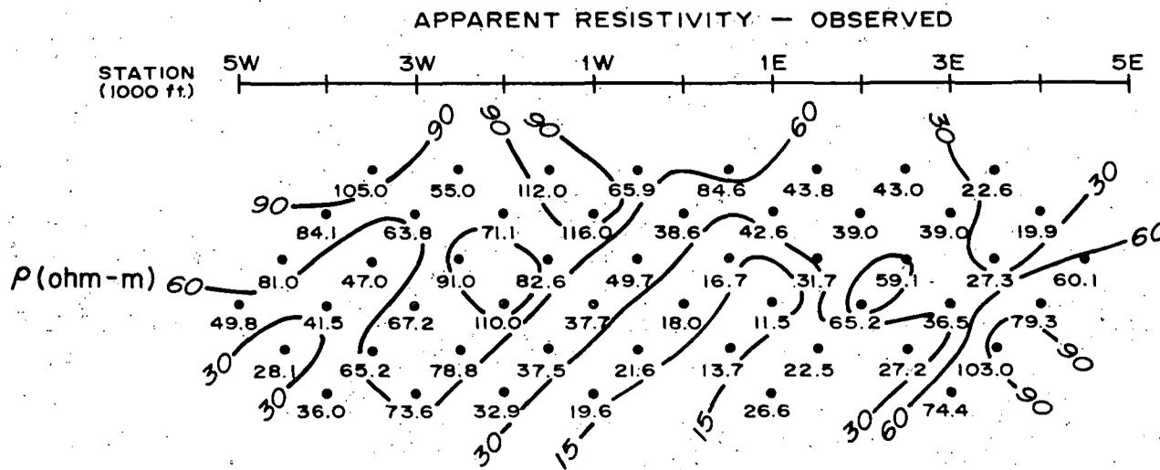
FIGURE 9 INTERPRETED RESISTIVITY SECTION AND OBSERVED APPARENT RESISTIVITY
