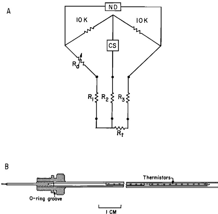
Fig. 1. (a)  $R_t$ , thermistor;  $R_1$ ,  $R_2$ , and  $R_3$ , lead resistances;  $R_d$ , 6-decade variable resistor; CS, current source (1.35-volt mercury cell with voltage divider); ND, battery-operated null detector. (Redrawn from Roy et al. [1968b].) (b) Sketch of thermistor probe.
