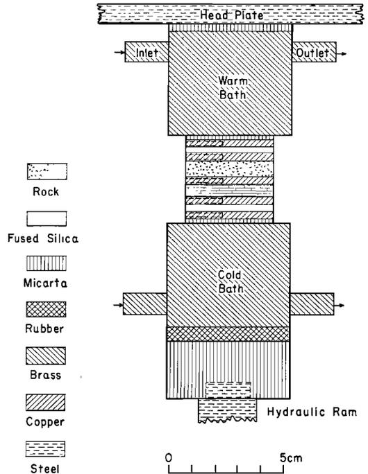
Fig. 2. Schematic representation of the divided-bar apparatus. The dashed lines in the copper sections are projections of cylindrical thermistor wells.
