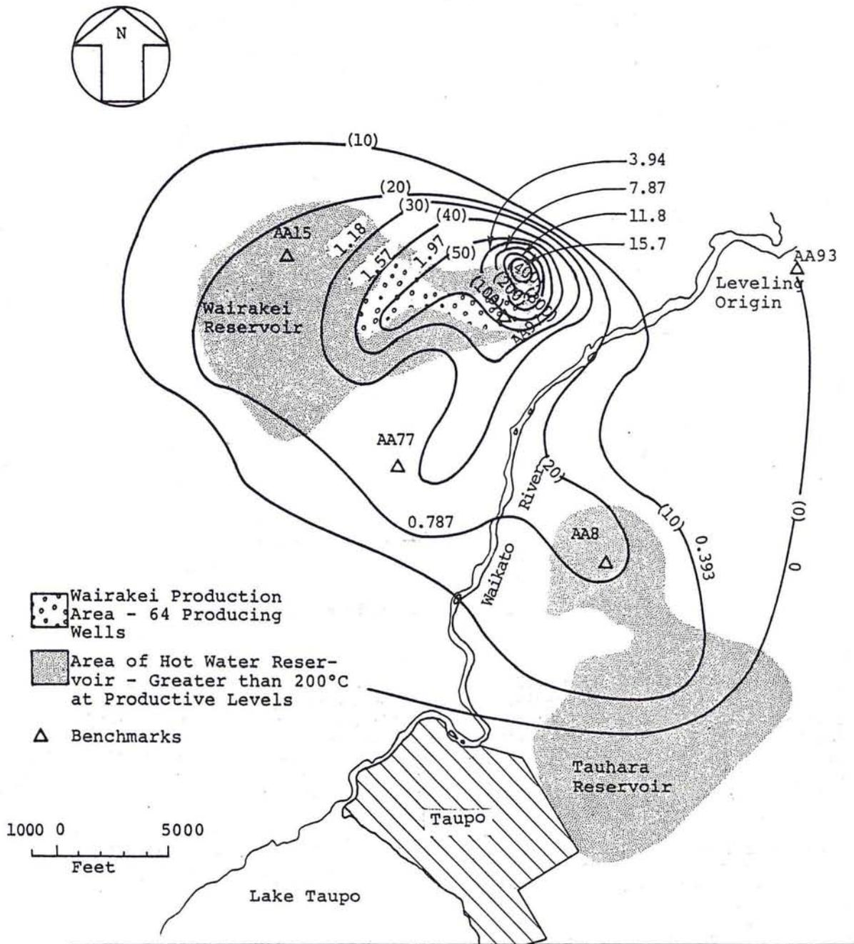
Figure 16. Average land subsidence rates, 1956-1971. Contours of equal subsidence in inches per year. Values in parenthesis are millimeters per year.
