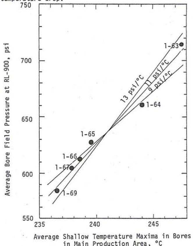
Figure 7. Average bore field pressure at RL-900 versus average maximum bore temperatures; temporal trend.
