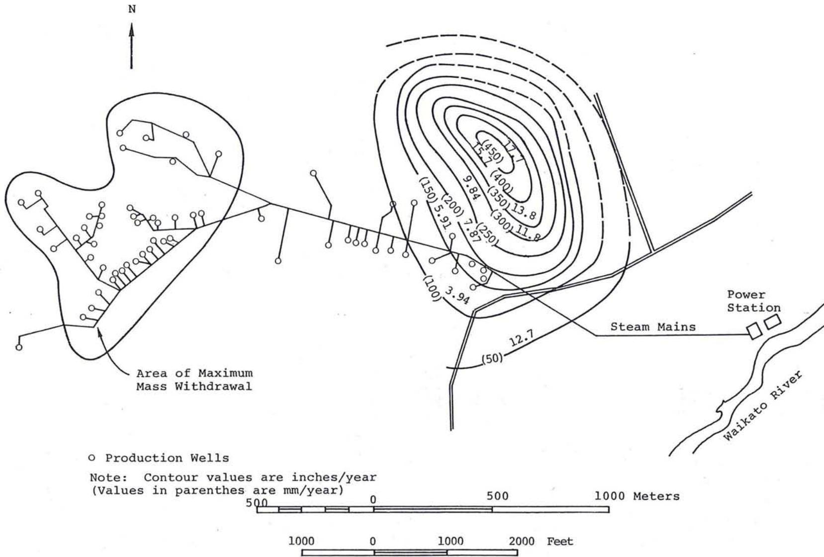
Figure 18. Subsidence rate in Wairakei production field 1964-1974.<sup>41</sup>
