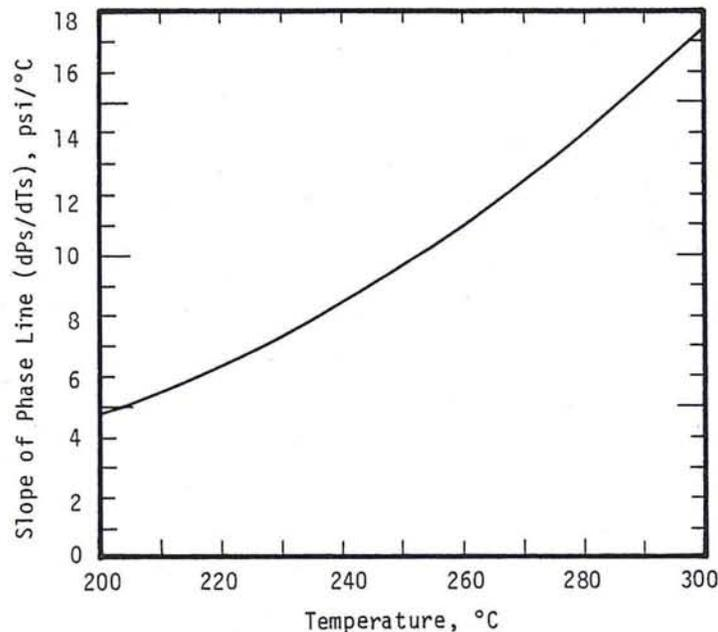
Figure 8. Slope of phase line versus temperature.
