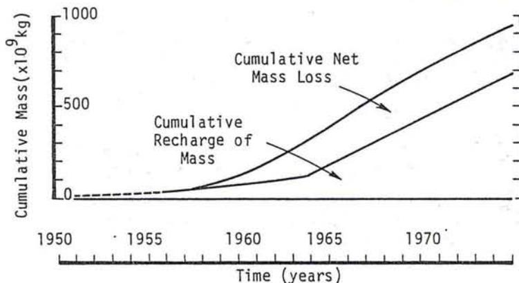
Figure 15. Cumulative recharge and cumulative net mass loss, estimated from corrected gravity differences at benchmark A97, Wairakei Geothermal Field.<sup>37</sup>
