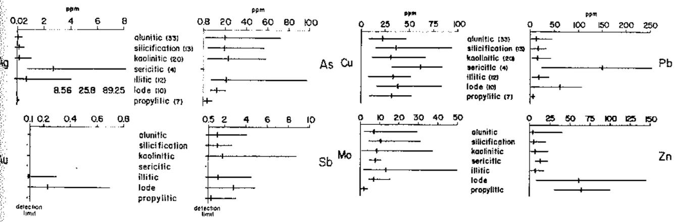
Figure 4. Graphs showing range of geochemical values (length of bar) and average values (crossbar) for various alteration assemblages from the Comstock district. Number in parentheses next to alteration assemblage is number of samples. Lode refers to lode material.
