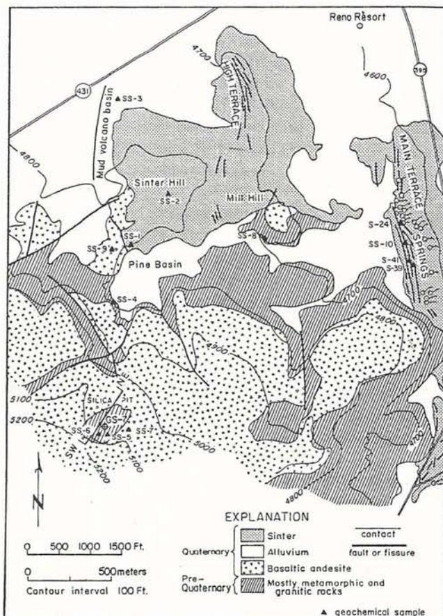
Figure 1. Generalized geologic map of the Steamboat Springs geothermal area, Nevada (redrawn from Schoen and others, 1974) showing geochemical sample locations for table 1.
