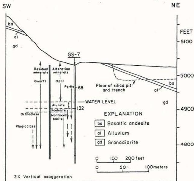
Figure 3. Geologic cross section of the Silica Pit showing wall-rock alteration in core from drill hole GS-7 (redrawn from Schoen and others, 1974, fig. 3).
