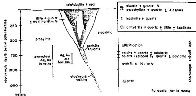
Figure 3. Restored diagrammatic west-east cross section of the Comstock Lode or one of its branches showing the approximate distribution of alteration and mineralization.
