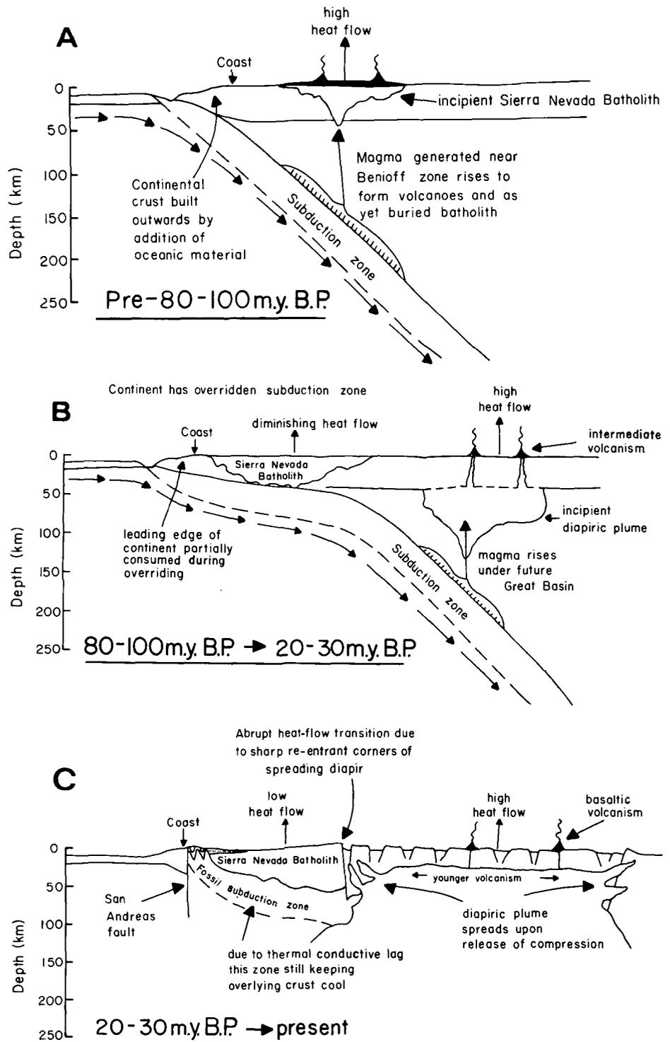
Figure 8. Schematic sequential representations of the Sierra Nevada-Basin and Range geothermal regime from the time of batholithic emplacement to the present.
