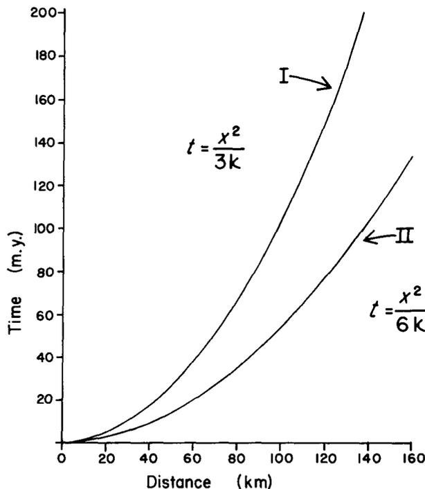
Figure 7. Examples of time  $t$  required for the heat flow at a distance  $x$  from a planar heat source to reach a maximum ( $k = 0.01$  cgs). Case I: continuous source imbedded in an infinite medium; case II: instantaneous source at depth  $x$  below the surface of a semi-infinite medium with zero surface temperature. Heat flow observed at surface.
