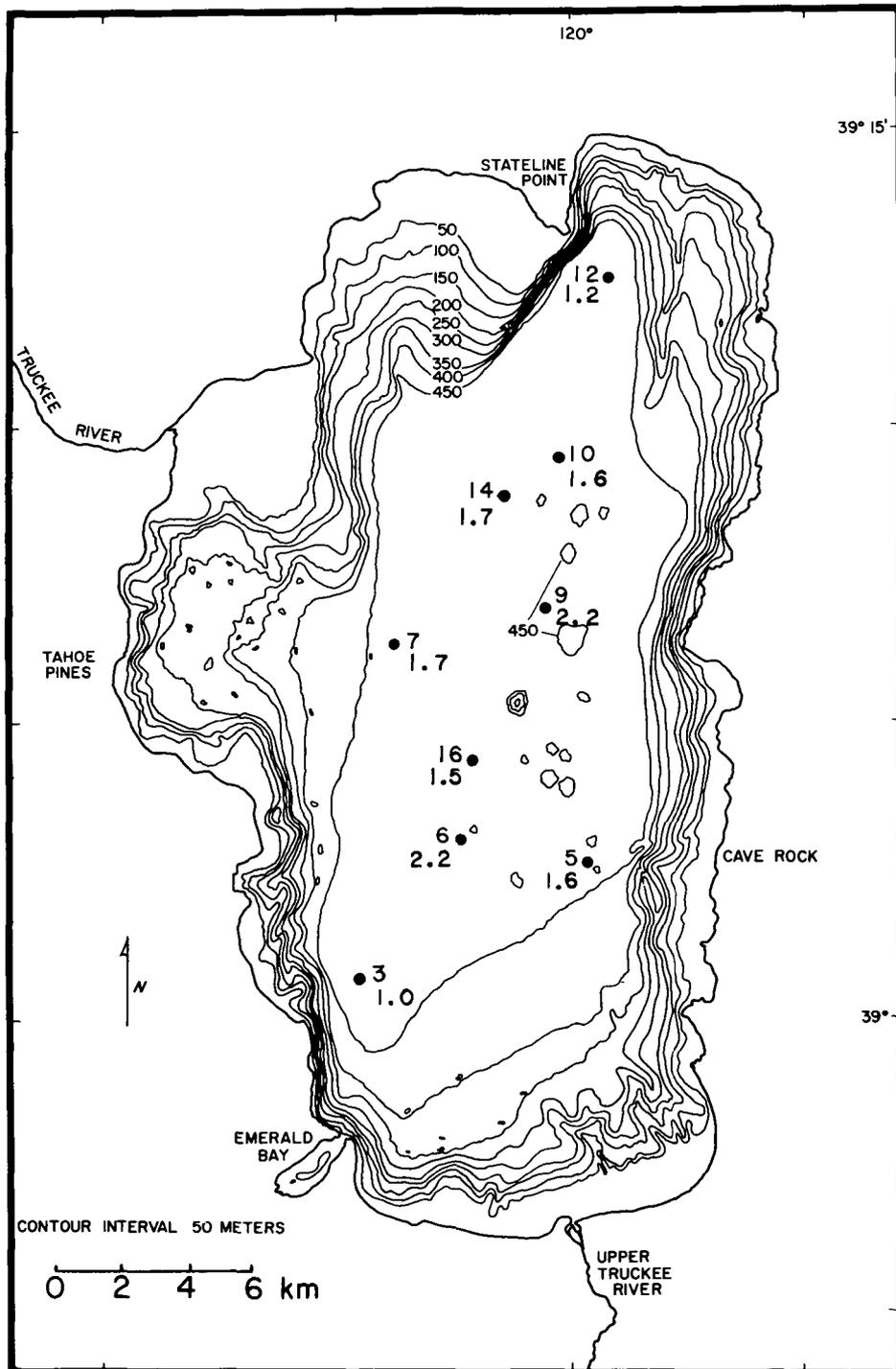
Figure 2. Bathymetry and locations of heat-flow stations, Lake Tahoe. Number on top identifies the station; number on bottom is the heat-flow value in  $\mu\text{cal}/\text{cm}^2/\text{sec}$ .
