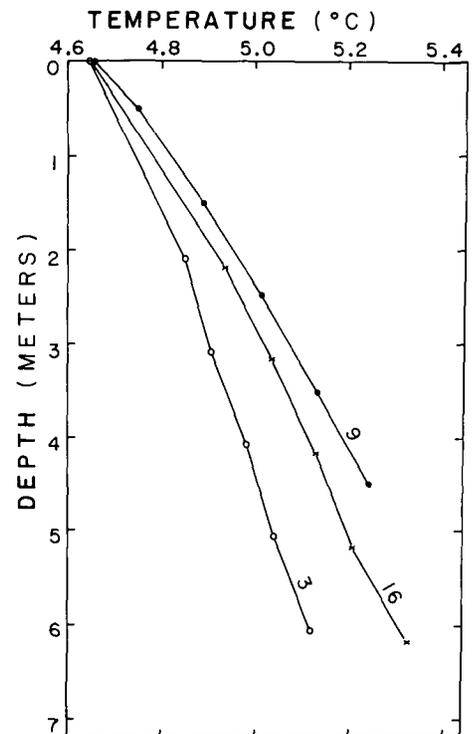
Figure 5. Three typical geothermal profiles from Lake Tahoe (from stations 3, 9, and 16).
