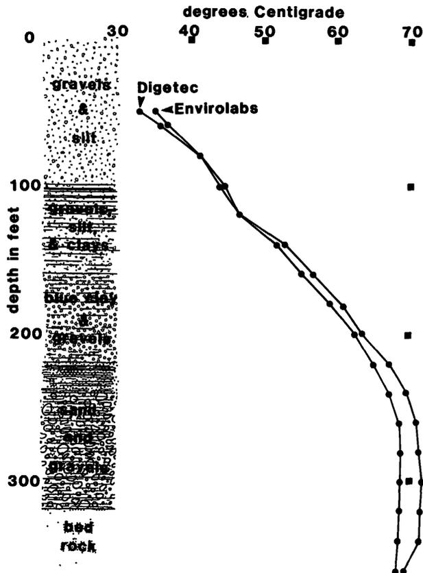
Figure 2. Lithologic log and temperature depth profile for Kemp 110 m (360 ft.) temperature gradient hole.
