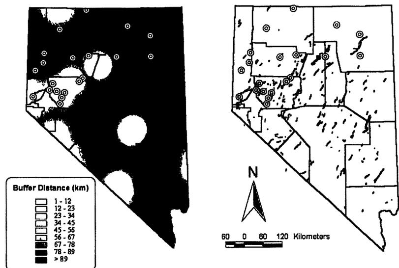
**Figure 1.** Distribution of high temperature (>160°C) geothermal systems (double circles) relative to (a) buffer distance to the nearest volcanic vent (<1.5Ma), and (b) northeast-striking faults (azimuths of 17-107 deg.) of late Pleistocene and younger age.
