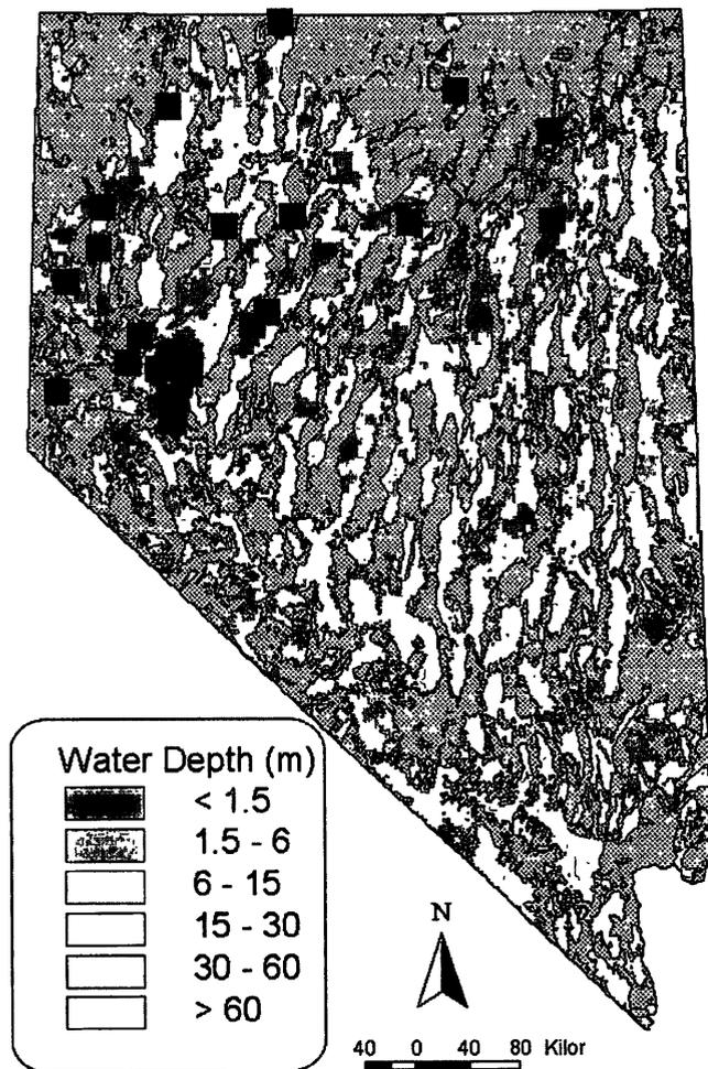
**Figure 5.** Depth to groundwater in Nevada, based on the USGS NWIS database. The background dotted pattern represents areas of "No Data", which are areas of non-Quaternary sedimentary rocks, occurring mostly in mountain ranges. Black squares are high temperature geothermal systems (>160°C).
