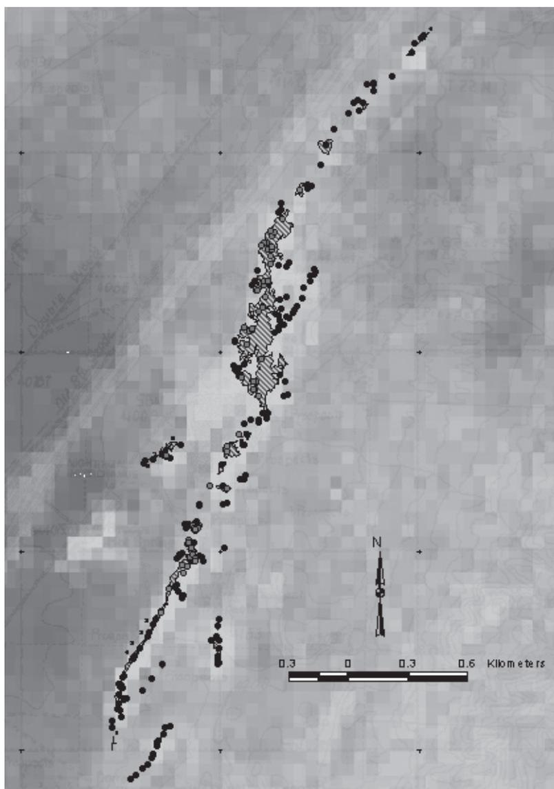
**Figure 5.** Thermal features at Bradys Hot Springs, Churchill County, Nevada, mapped with a hand-held GPS unit. Black dots are warm ground, gray dots are mud pots and loud steam vents, and striped polygons are larger areas of warm ground. Lighter-colored background areas represent temperature anomalies detected with nighttime Landsat and ASTER thermal infrared imagery.
