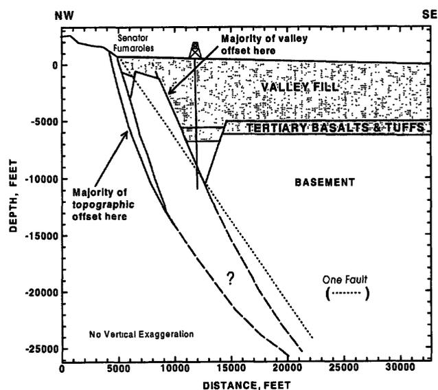
**Figure 6.** Fault splay model of the Dixie Valley/Stillwater Range bounding structure compared to the single fault model.
