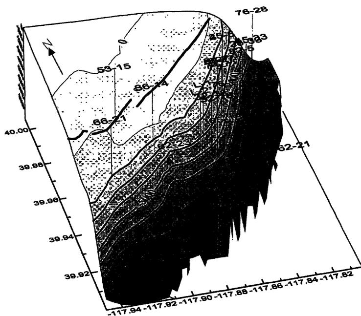
**Figure 5.** Perspective diagram of the range/valley contact with the valley fill removed. The depths have been calculated and contoured based on a density contrast of  $-0.5 \text{ gm/cm}^3$  from profiles like those shown in Figure 4. Well locations are also shown.
