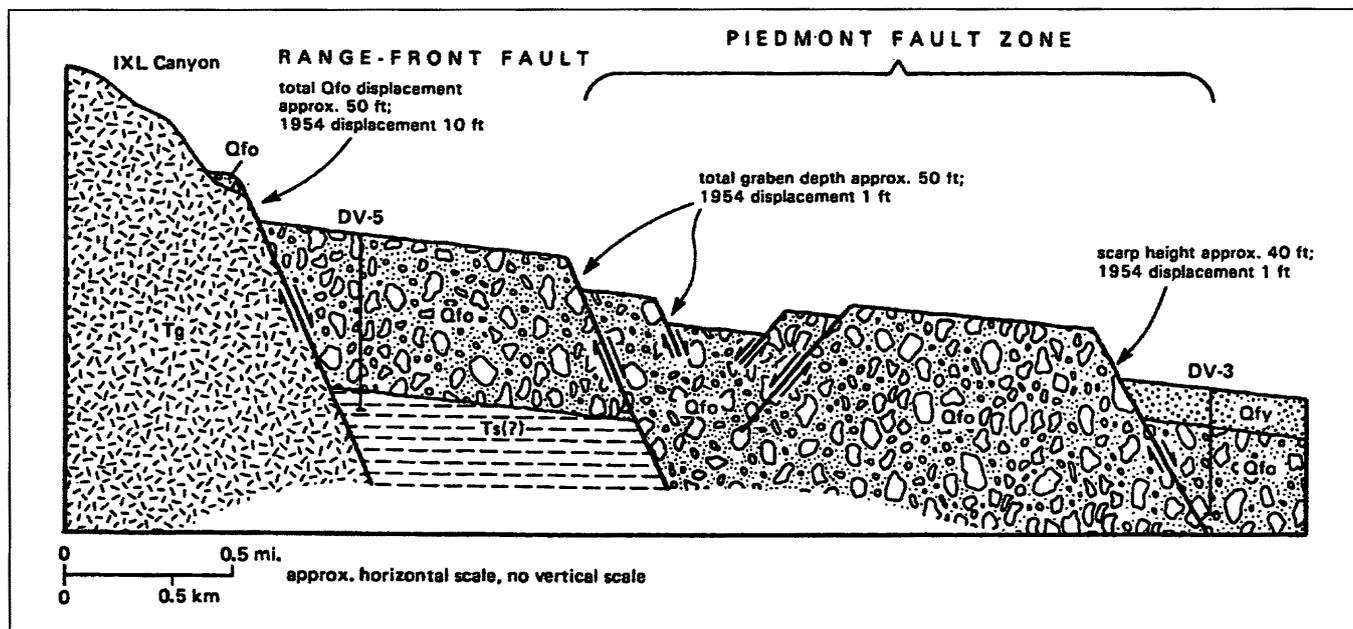
Figure 7. Schematic composite cross section of the IXL and East Job Canyons range-front and piedmont faults. Tg: Tertiary granite and granodiorite; Ts: Tertiary sediments; Qfo: old alluvial-fan deposits; Qfy: young alluvial fan deposits (from Bell and Katzer, 1987, Figure 37).
