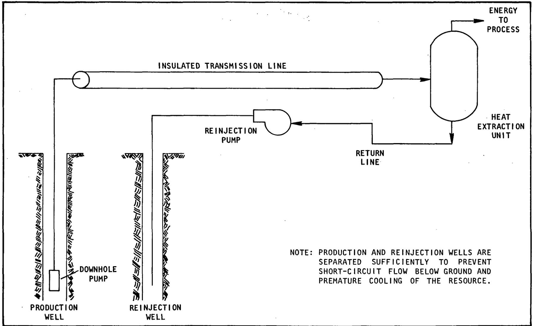
Figure 1.--Geothermal direct use energy system.
