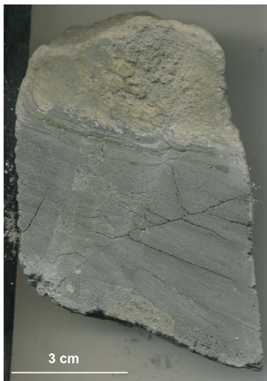
Figure 14. (a) Cut core sample AX46-1268 of CSD mineralization hosted in the Panther Canyon dolomite submember. Sample is HQ core assaying 1.02 g/t Au and 1.5 g/t Ag.
