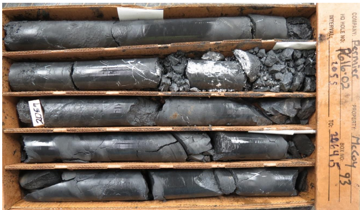
Figure 19. Core photo of PG16-02 at the Gap deposit, which is hosted in the informal middle unit of the Favret Formation. This core is part of an intercept of 50.9 m of 7.08 g/t Au. HQ core, units are in feet.
