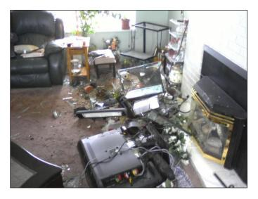
**Figure 11.** Content damage and dislocation that was typical of areas of intensity MMI VI (photo by resident).
