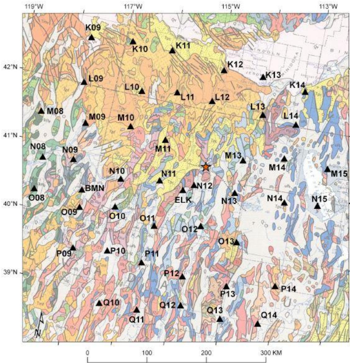
**Figure 1.** USArray and ANSS broadband stations (triangles) located within 300 km of the 2008 Wells, Nevada earthquake (star). The base map illustrates the geologic complexity of the seismic wave travel paths: light gray—Quaternary sediments; yellow—Tertiary continental deposits; orange—Tertiary volcanic rocks; green—Mesozoic volcanic and intrusive rocks; blue—Paleozoic volcanic and intrusive rocks. From Mendoza and Hartzell (2009).
