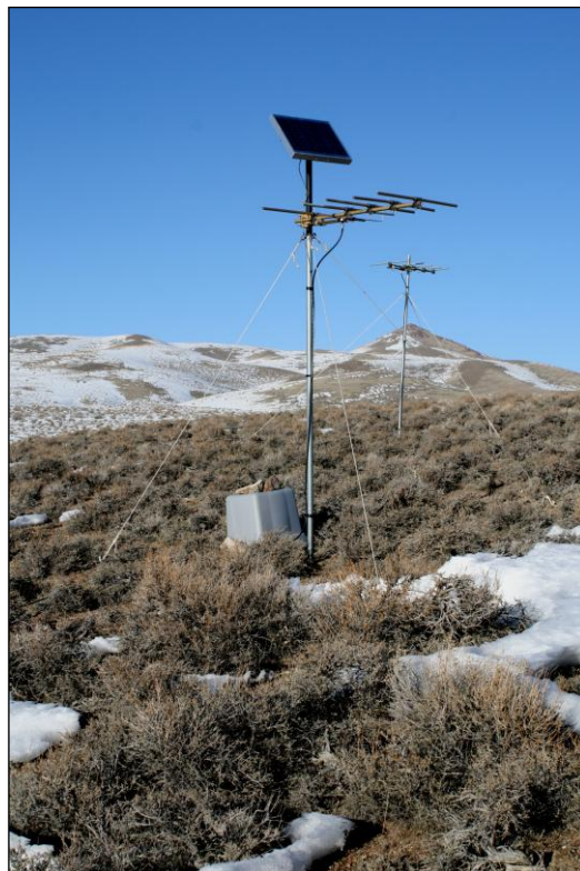
Figure 20. Temporary seismic array station with transmission antennas installed to record aftershocks from the Wells earthquake. These stations are used to precisely locate the aftershocks and also to provide the characteristics of ground motion at the site.
