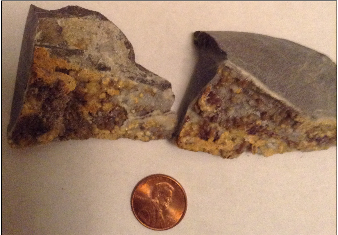
Fig. 41: Fracture in quartzite, coated with tan to red siderite.
