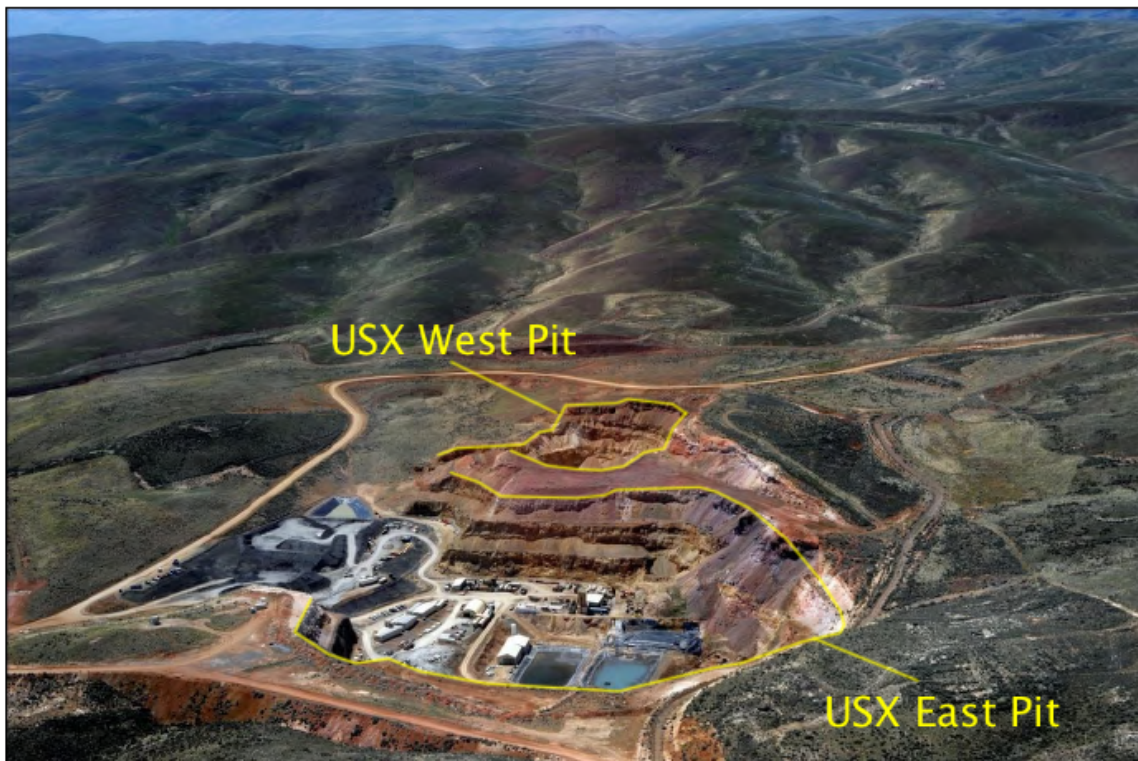
Fig. 3: Perspective view of the USX East and West pits, looking WSW. Modified from Oelofse et al., 2011. Buried vein systems are to the right of the open pits and off the photograph.
