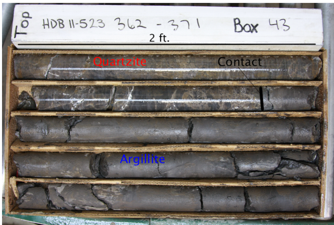
Fig. 9: Drill core showing quartzite and argillite of the Vinini Formation.
