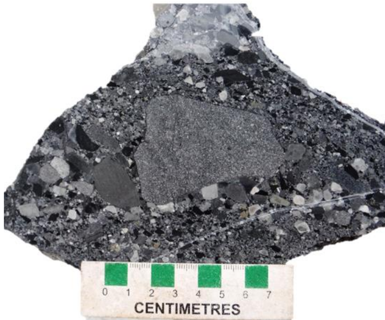
Fig. 3.18. Hand sample displaying a poorly sorted sedimentary heterolithic breccia (BxS).
