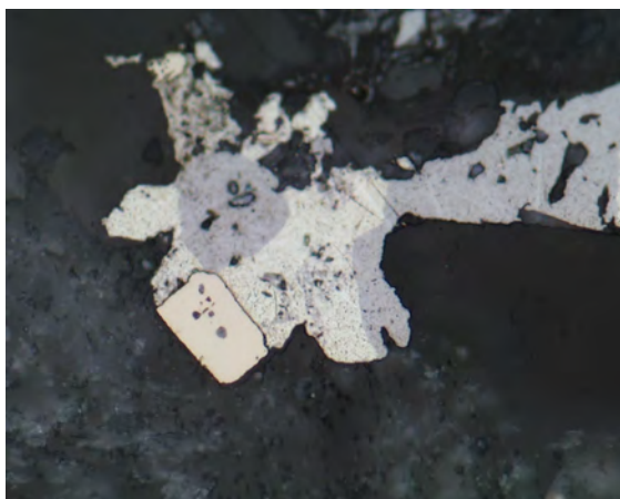
21) Tennantite intergrown with galena rimming/intergrown with pyrite. FOV= 0.16 mm; Sample 44, 3362 ft.
