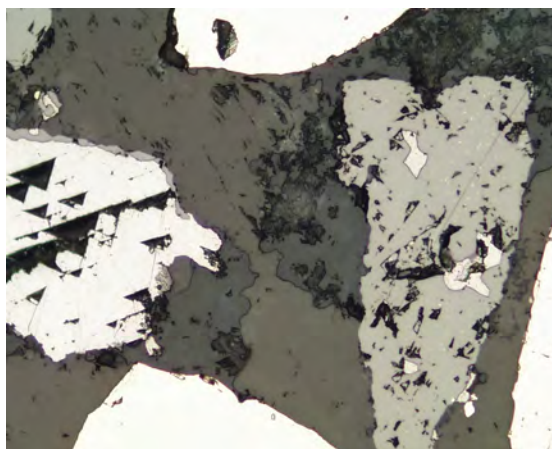
6) Galena intergrown with sphalerite (high Fe, chalcopyrite disease) and rimmed by sphalerite (high Fe, no chalcopyrite disease). FOV= 0.43 mm; Sample 44, 3362 ft.
