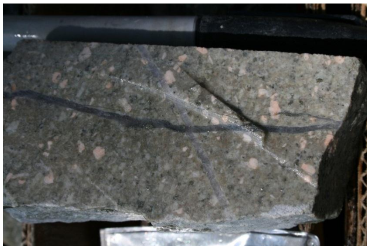
Figure 30: Photograph of a planar crack-seal quartz-pyrite vein (white) crosscut by an irregular gray quartz-tourmaline-pyrite vein in the Feldspar Porphyry. Further down hole, the white crack-seal vein is also crosscut by a 6-8mm planar gray quartz-pyrite-carbonate vein. Core is 2.5 inches in diameter.
