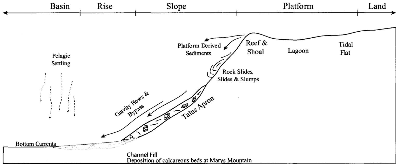
Figure 25. Generalized carbonate platform-slope-basin showing deposition of calcareous material as turbidites deposited along the toe of the slope and as channel fills in the deeper parts of the basin (modified from Cook, 1983).
