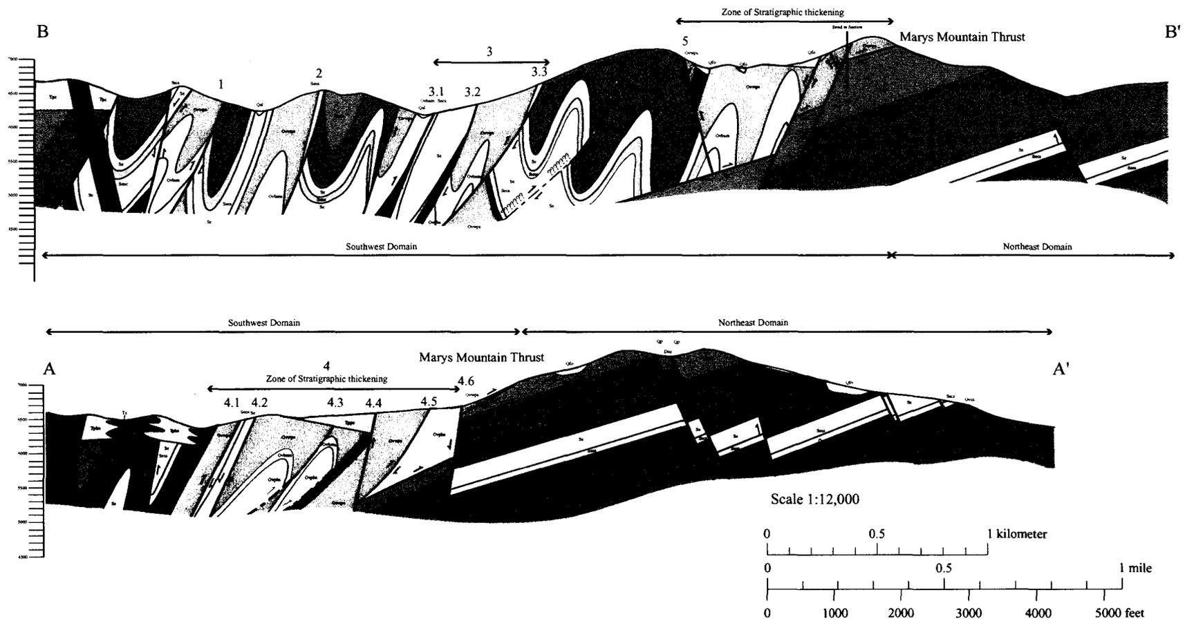
Figure 21. Cross section of the Marys Mountain area. Although the isoclinal folds and imbricate reverse thrust faults were inferred by Henry and Faulds (1999), the biostratigraphic work permitted the precise location of many of the faults and folds. Locations of cross sections are shown on Plate 1.
