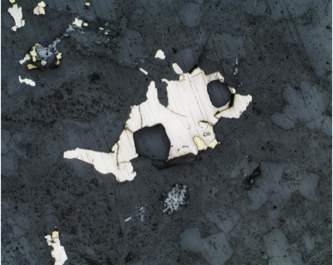
Figure D-16. Disseminated pyrite grain showing replacement by chalcopyrite. Reflected light, field of view = 0.85 mm.
