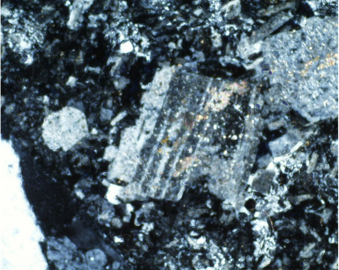
Figure D-12. Plagioclase phenocryst with weak calcite replacement. Cross-polarized light, field of view = 1.7 mm.
