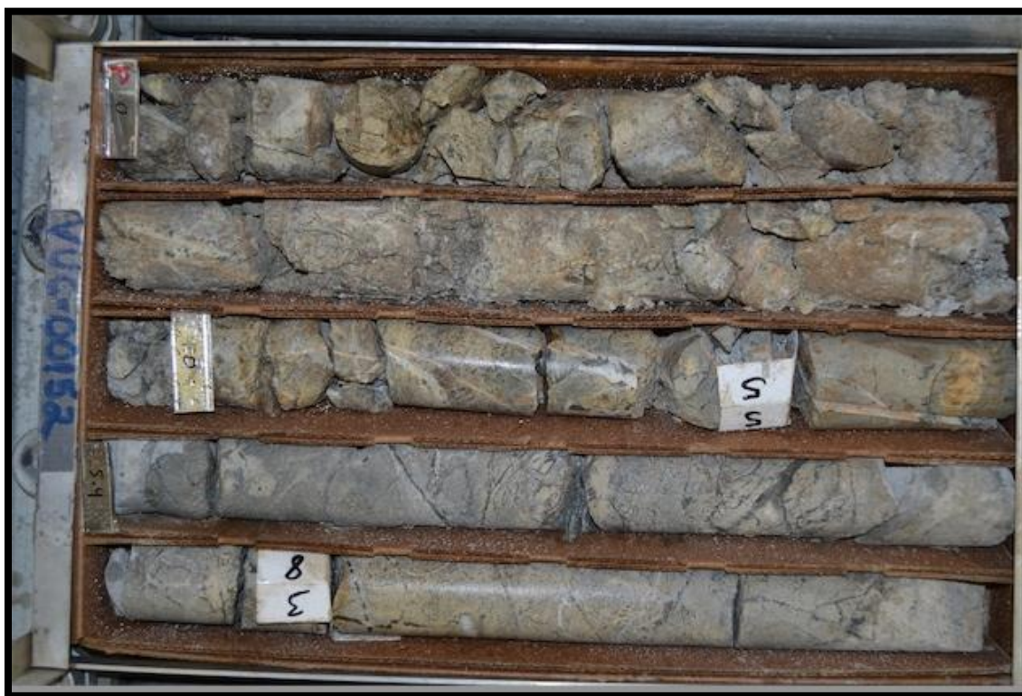
Figure 45. Core box photograph from VUC-00152 of argillic altered basalt.
