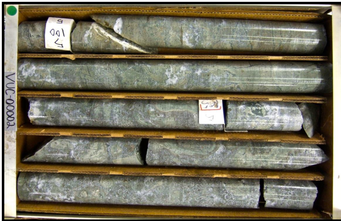
Figure 11. Core box photograph from VUC-00002 of a flow breccia.
