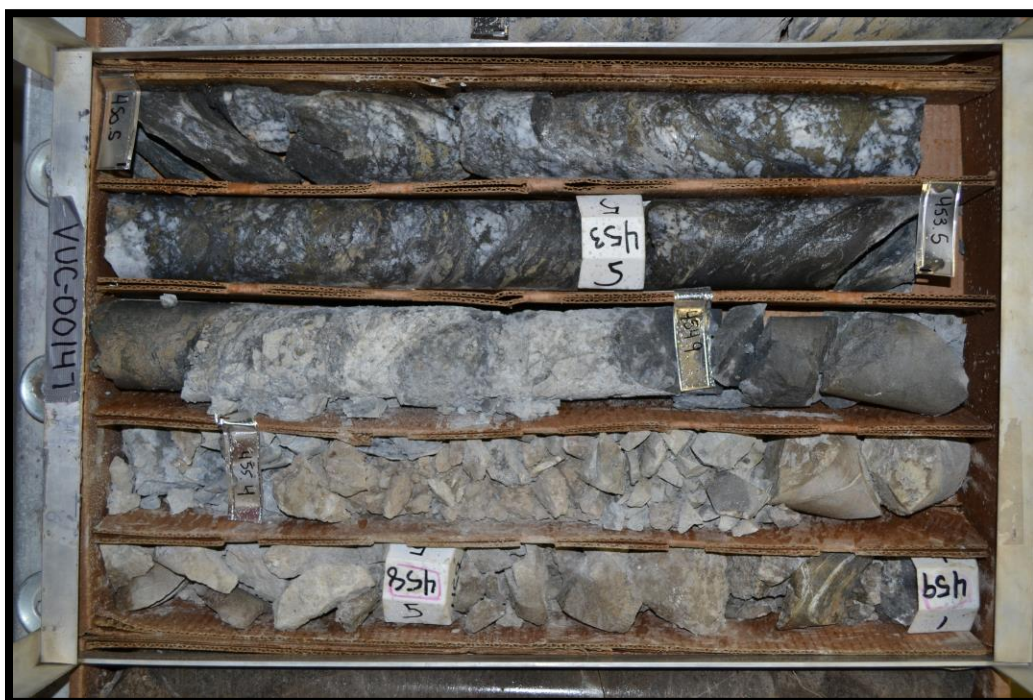
Figure 22. Core box photograph of the Galena Vein in VUC-00147. The Galena Vein is from 450.5 - 453.5 ft. The gold assay for this interval is 1.01 oz/ton. The core box is two feet long.
