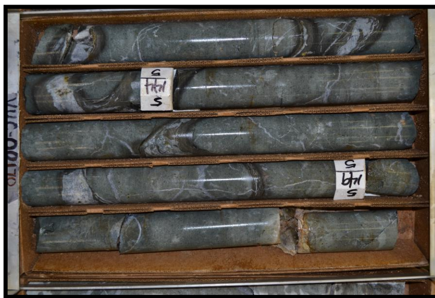
Figure 8. Core box photograph from VUC-00170 of propylitically altered pillow basalt.
