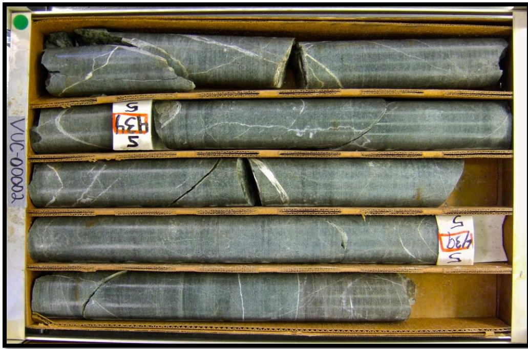
Figure 9. Core box photograph from VUC-00002 of propylitically altered massive basalt.
