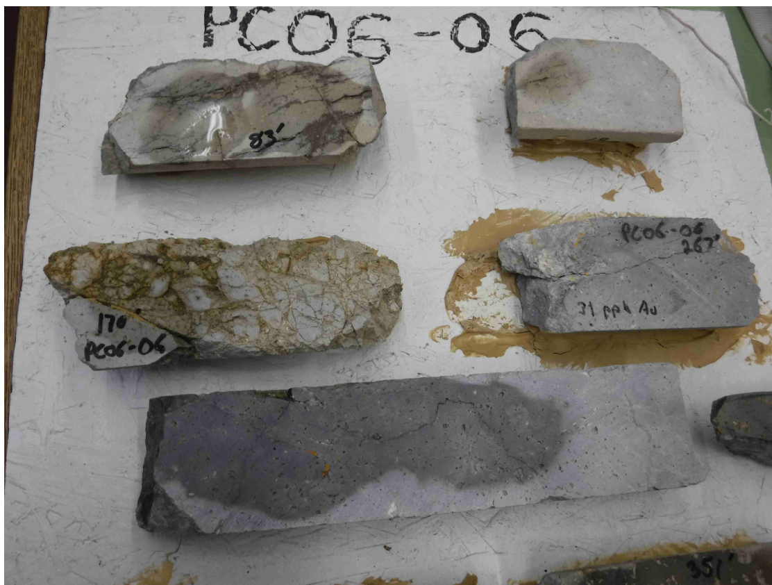
Figure 12.1. Core from drillhole PC06-06 drilled in 2006 at the Bowl Zone showing the porphyritic rhyolite geological unit and a brecciated interval of intense faulting.
