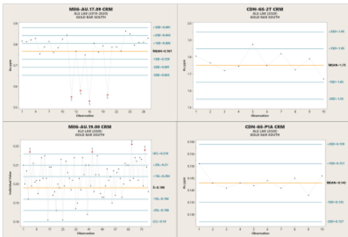
Figure 11-8: Graphical Representation of CRM Results in Chronological Order. Mean Au Value is Represented by the Orange Line with 1, 2, and 3 Sigma Lines Presented in Blue (McEwen, 2020).
