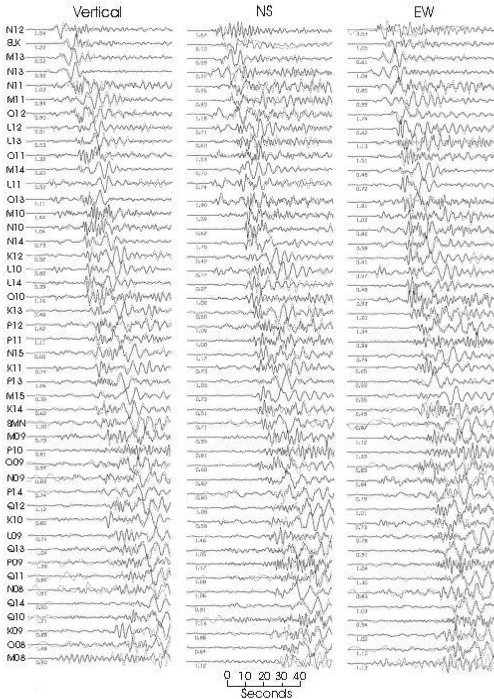
**Figure 4.** Observed (solid) and predicted (dotted) vertical, north-south (NS), and east-west (EW) bandpass-filtered velocity records for the source model inferred by Mendoza and Hartzell (2009) for the 2008 Wells earthquake. Records are shown in order of increasing epicentral distance from top to bottom with numbers indicating the ratio of predicted-to-observed amplitudes.
