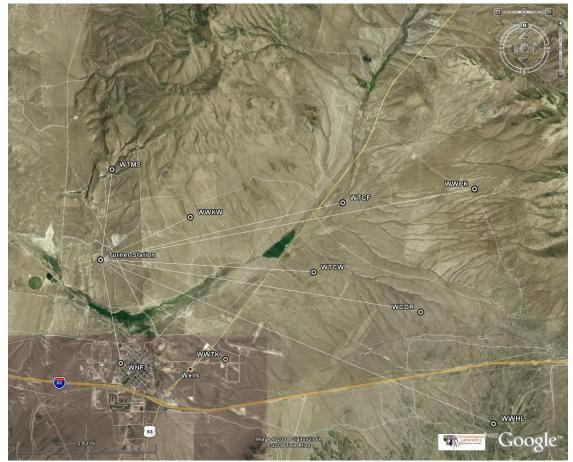
Figure 3. Map of telemetry paths for USGS RT130 instruments to DoIT relay Turner Station (map using software application Google Earth <a href="http://earth.google.com/">http://earth.google.com/</a>).
