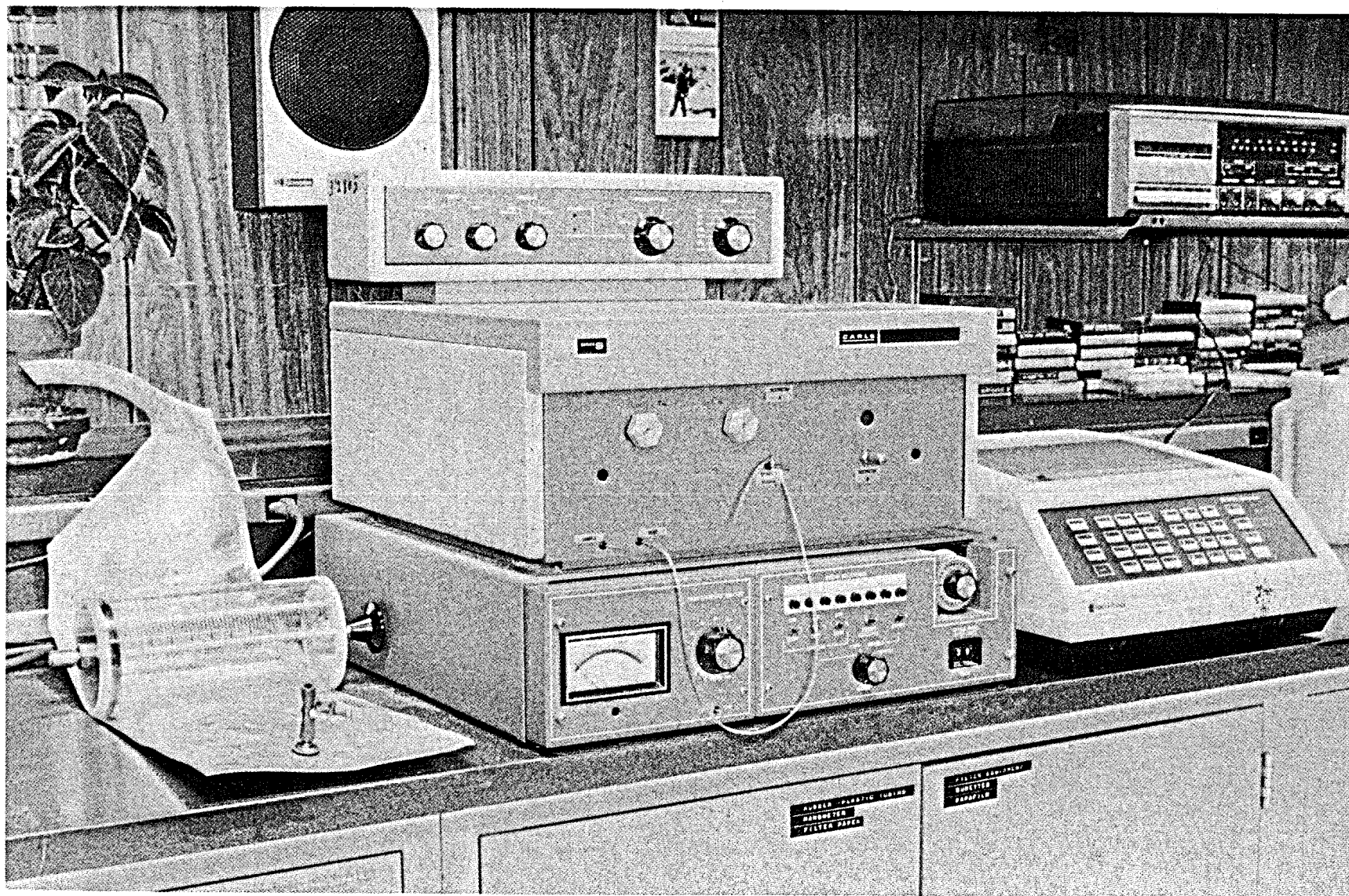
Fig. 17. Carle Model 111 H Gas Chromatograph.
