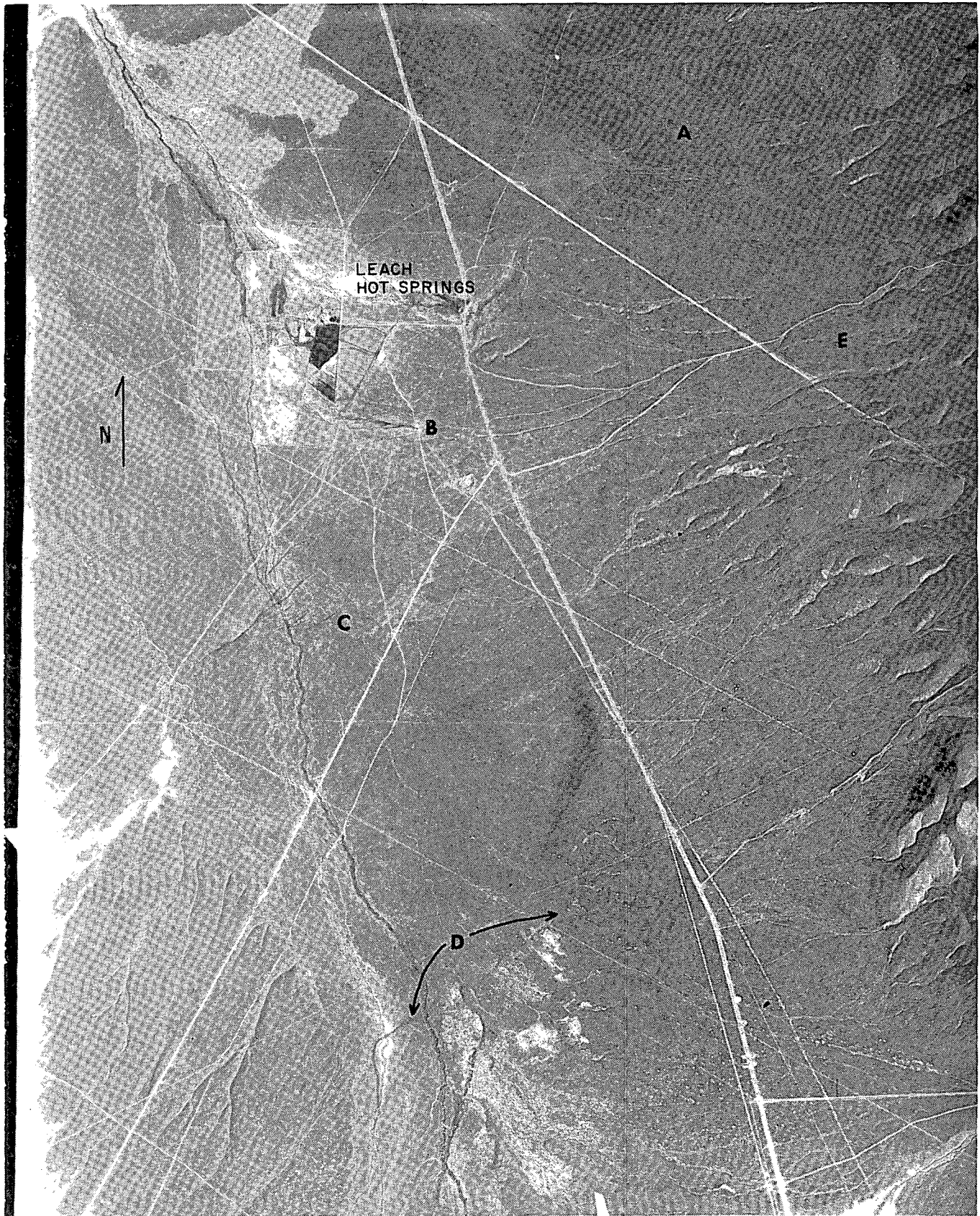
FIGURE 12. Low sun-angle aerial photograph of the Leach Hot Springs area showing northeast trending faults in alluvium. The hot springs are located along scarp A. Another spring B is located along strike between the main hot springs A and a series of northeast trending fractures at C (scale 1:30,000).
