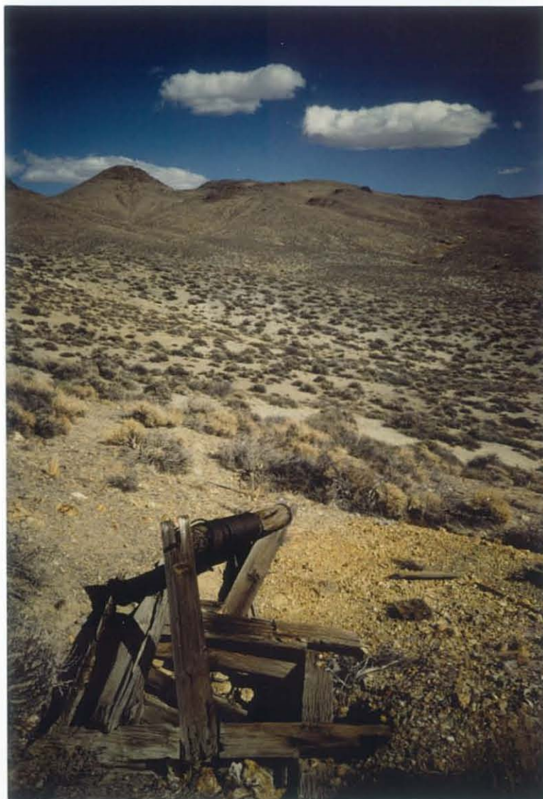
Photo 7-9 Remains of hand windlass over shaft at sample site 5538, Antelope Springs district ( J. Tingley photo ).
