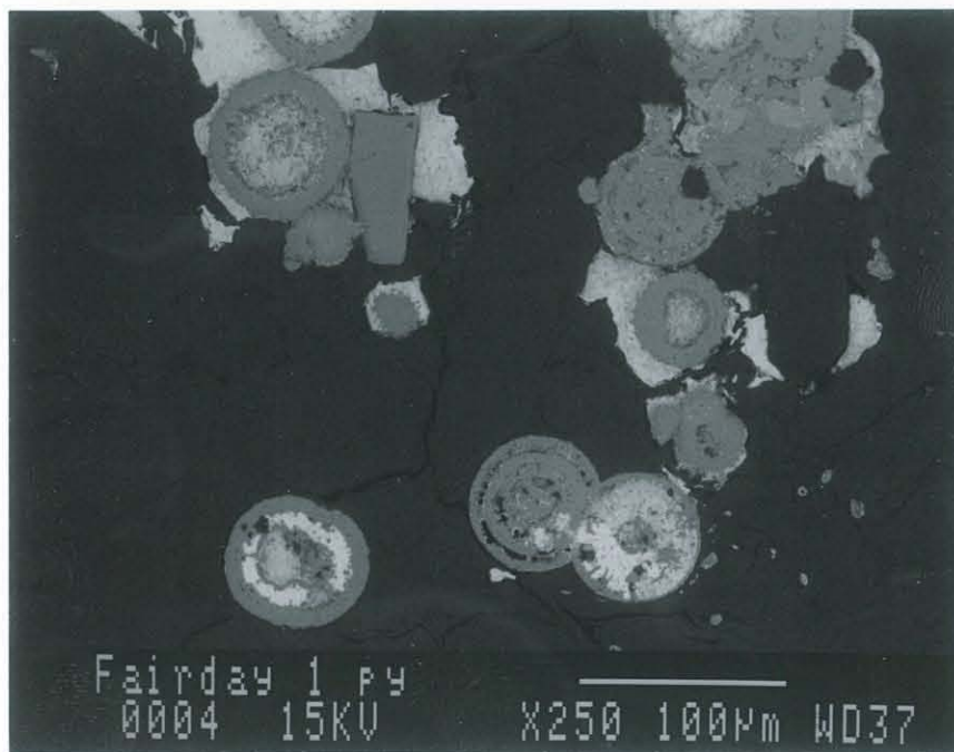
Photo 7-16 Back-scatter electron image of ore minerals from the Fairday Mine, Cactus Springs district, showing spherical grains composed of pyrite, galena, and a silver-bearing telluride mineral ( L. Christensen photo ).
