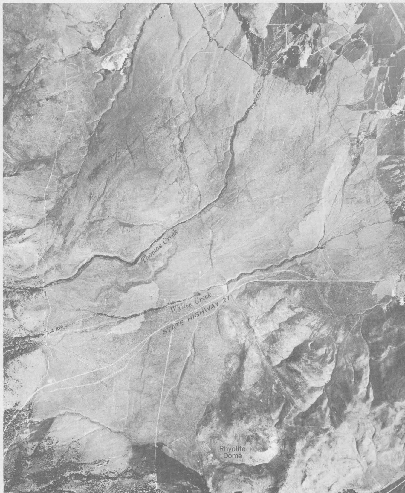
FIGURE 16.—Vertical aerial photograph showing swarms of en echelon fault scarps cutting alluvium west and north of Steamboat Hills. Width of photograph 4 miles; north is at the top. The two conspicuous creeks are Thomas and Whites; Steamboat Hills in southeastern part of photograph.
