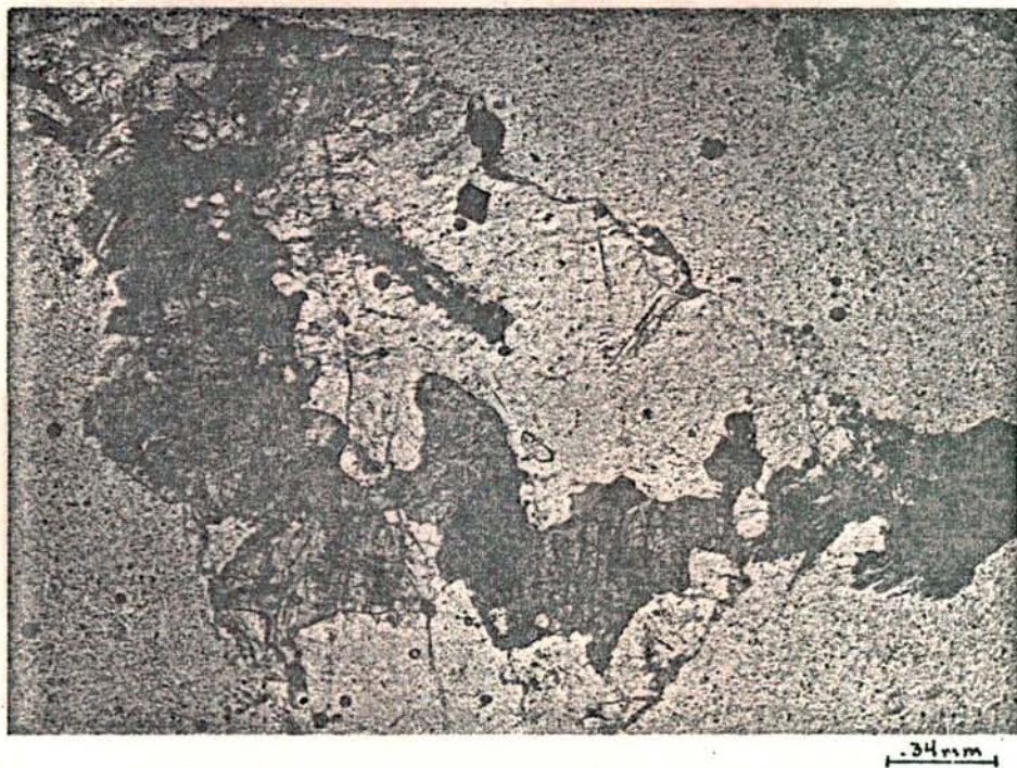
Figure 30. Same as Figure 29 without crossed polars. Note clarity of plagioclase crystal.
