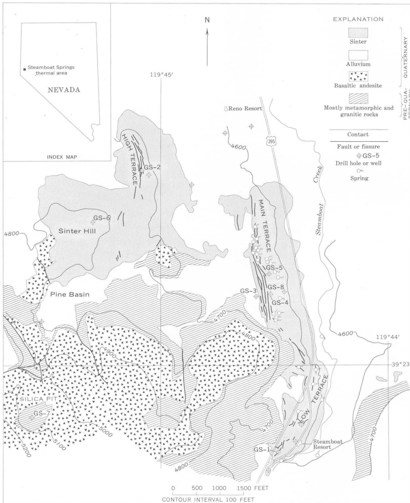
FIGURE 1.—Generalized geologic map of Steamboat Springs thermal area, Washoe County, Nev. (Modified from detailed map, White and others, 1964.)
