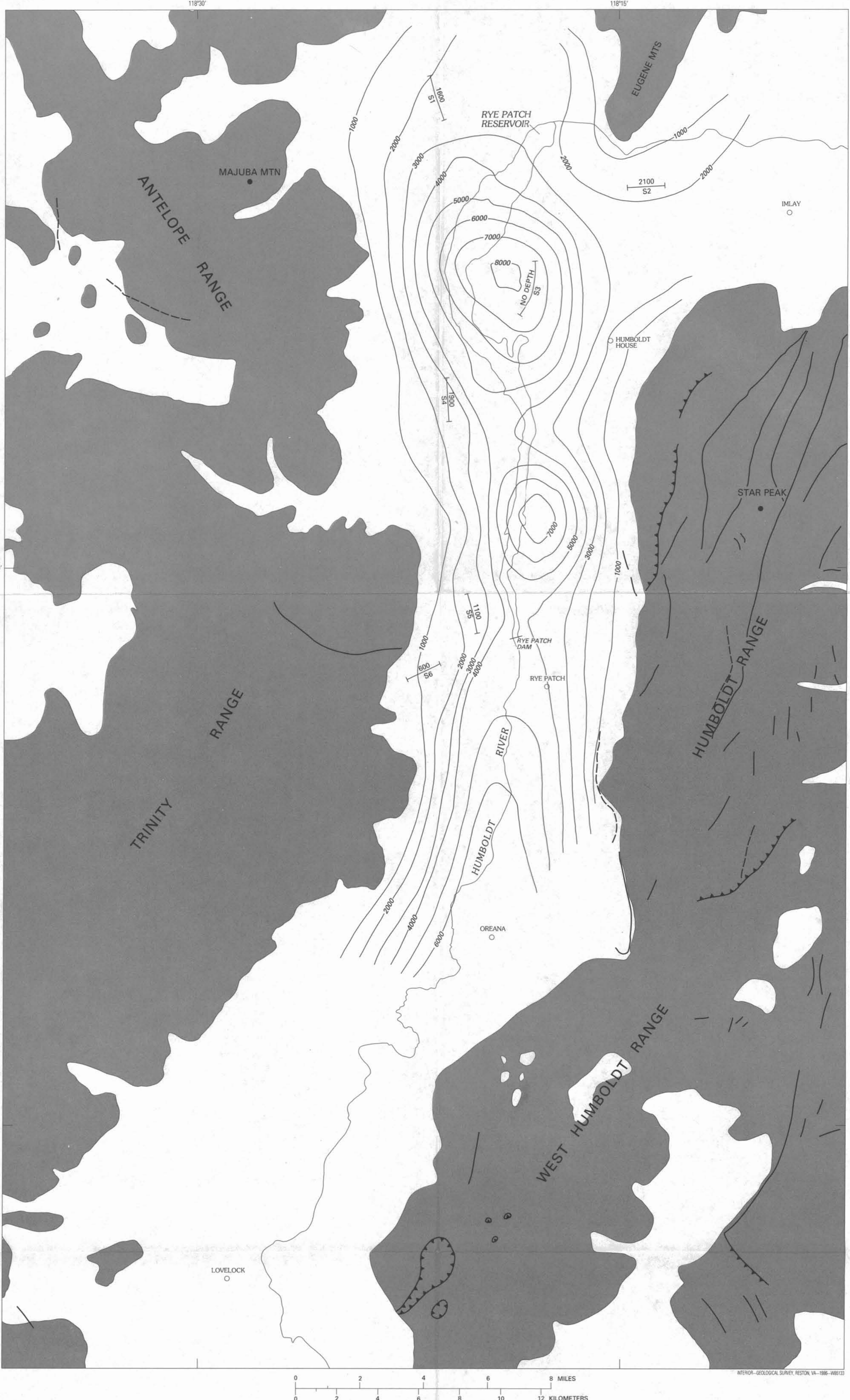
FIGURE 3—Depth to bedrock and location of seismic refraction lines.
