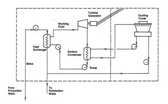
FIGURE C-3 Schematic Diagram of a Binary Cycle System.
