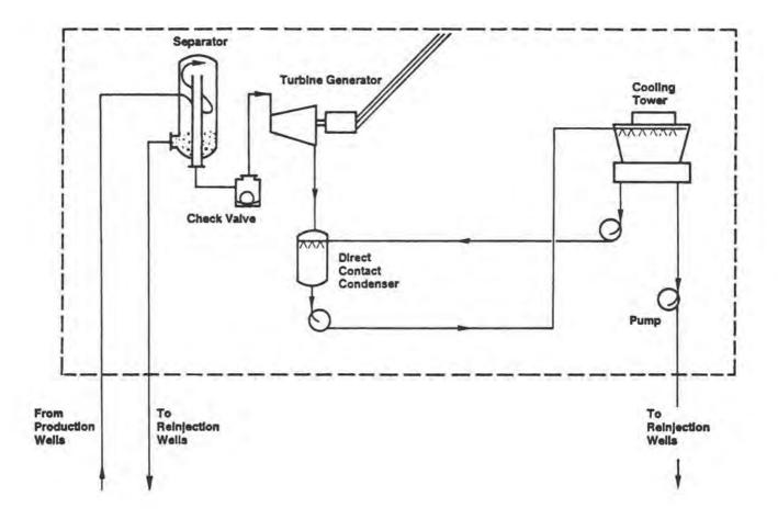
FIGURE C-2 Schematic Diagram of a Single Flash System.
