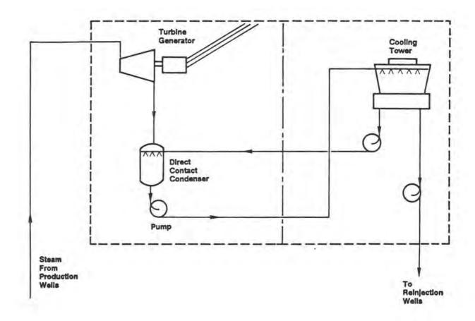
FIGURE C-1 Schematic Diagram of a Dry Steam System.
