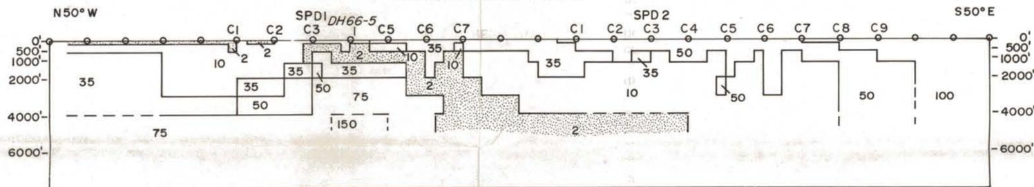
OBSERVED APPARENT RESISTIVITY (ohm-meters)
