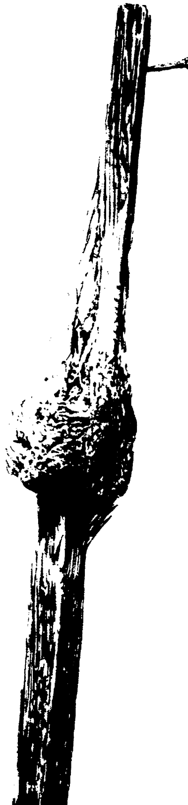
FIGURE 15.—Wood post shattered by salt, an example of evaporation effects on the saltpan. This wood post, 3½ feet long, was set in the flood plain of Salt Creek about 1910; ground level was at the lower edge of the bulge. Water rising in the wood evaporated at ground level and burst the wood with precipitated salts. Drawn by John R. Stacy, from photograph.
