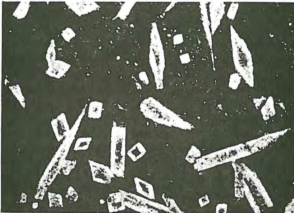
Figure 4-4. (b) Photomicrograph of andalusite/chiastolite crystals in very organic-rich metasilstone/metashale. (scale 13 mm : 0.34 mm)
