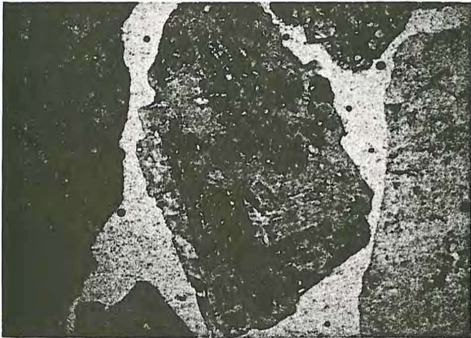
Figure 4-11. (b) Photomicrograph of epidote alteration in cores of plagioclase crystals. (scale 13 mm : 0.34 mm)
