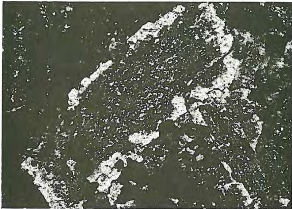
Figure 4-10. (b) Photomicrograph of sericitization confined to the core of a zoned plagioclase crystal. View under polarized light. (scale 13 mm : 0.27 mm)
