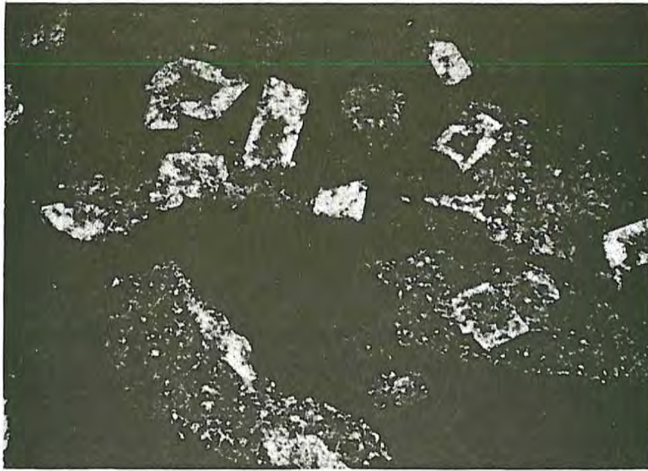
Figure 4-6. Photomicrograph of highly sericitized andalusite/cordierite porphyroblasts in metasilstone/metashale from DF 45-14 under polarized light. (scale 13 mm : 0.34 mm)
