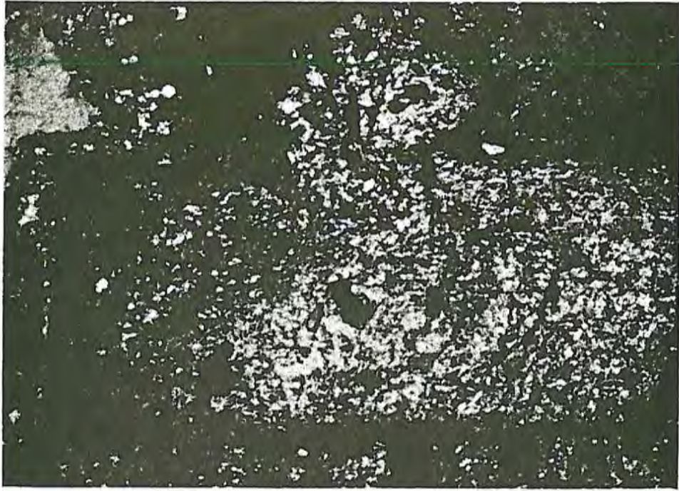
Figure 4-10. (a) Photomicrograph of a plagioclase crystal completely consumed by sericite. View under polarized light; note retention of crystal form. (scale 13 mm : 0.27 mm)
