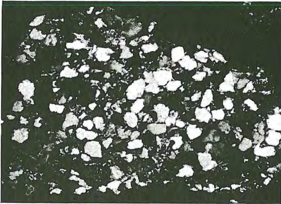
Figure 4-3. (a) Photomicrograph of metarenite facies under polarized light. (scale 13 mm : 0.22 mm)
