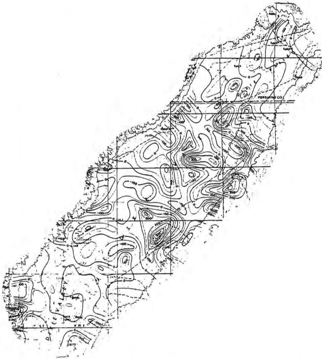
Figure 3-4. Second vertical derivative of aeromagnetic data for Dixie Valley. (from Smith, 1971)
