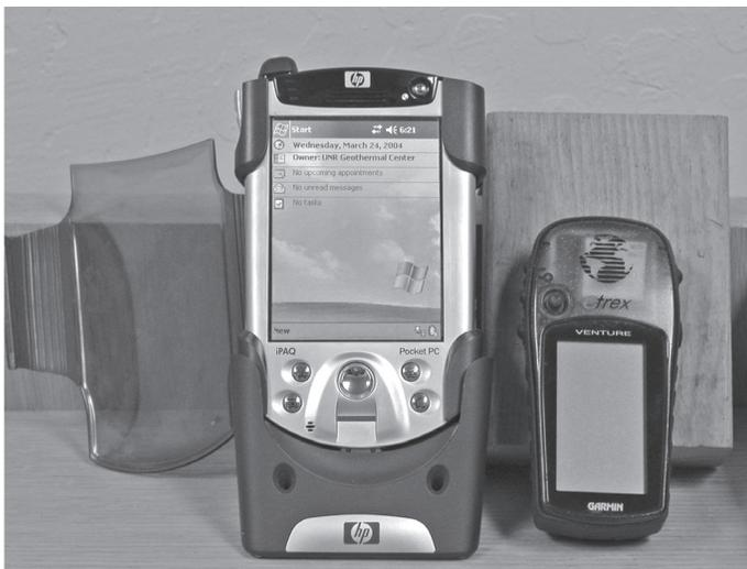
**Figure 1.** The HP hand-held iPAQ 5550<sup>®</sup> pocket PC (on left) and Garmin eTrex Venture<sup>®</sup> (right) used for mapping surface geothermal features.
