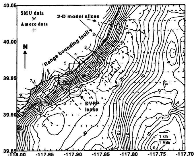
Figure 3. Complete Bouguer gravity residual-anomaly map and locations of sections in Figure 4. Gravity anomaly in mgal.
