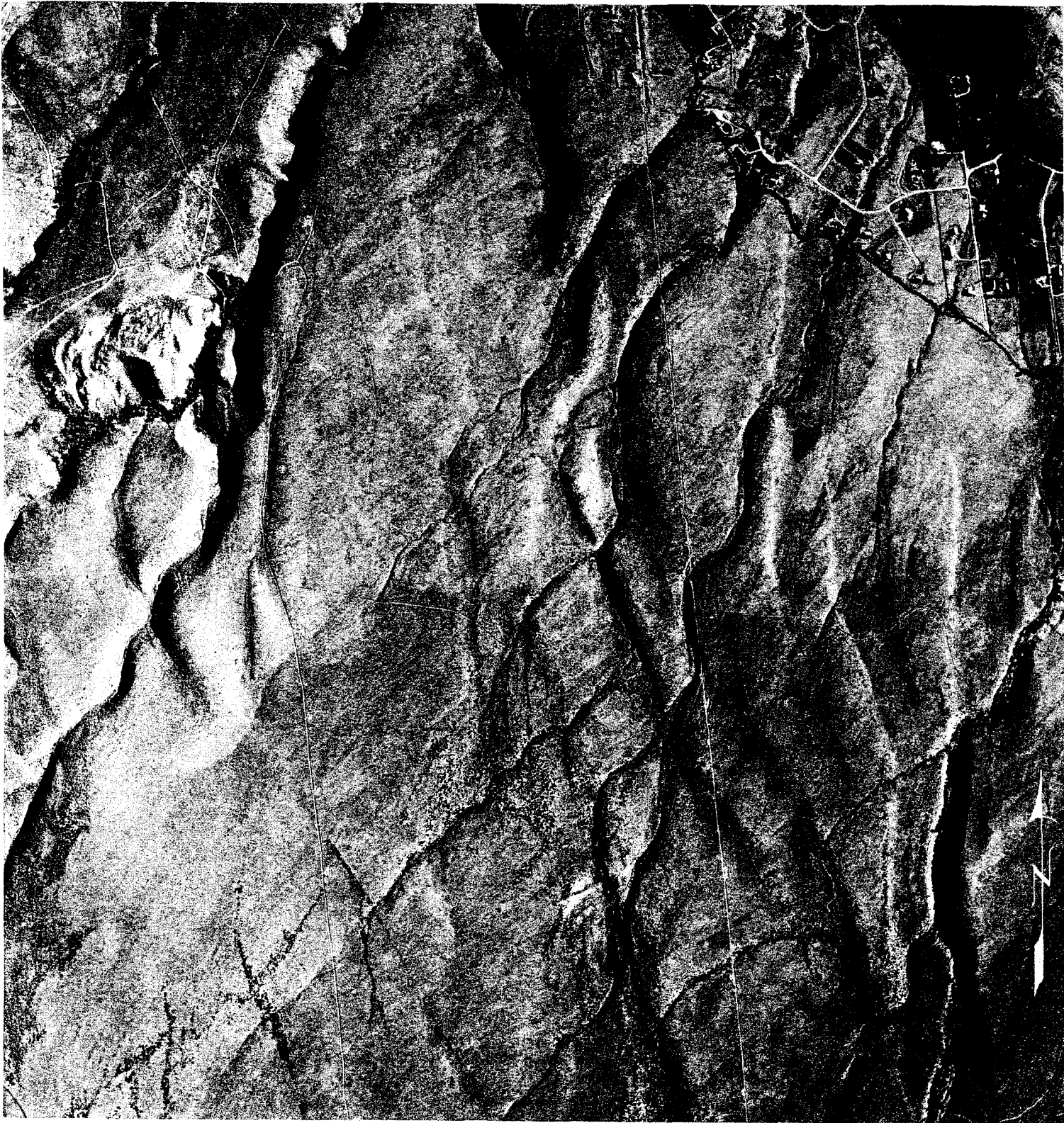
Densely faulted northeast margin of the Mount Rose fan complex. Here faults transect a thin veneer of Illinoian (?) pediment gravel resting on diatomaceous siltstone beds (sandstone of Hunter Creek). A landslide complex, seen as a light-colored patch along the left margin, includes both bedrock and pediment gravel.
