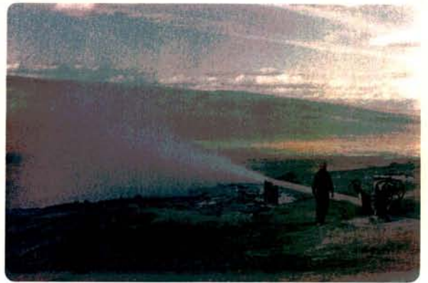
Figure 9. - Beowawe Geysers. Open Magma Power Co. Steam well. Mr. E. H. Hager at well head. Conductor pipe is 20-in., casing 13 3/8-in., with 8-in. gate valve and flow line. Steam jet is about 50 ft. long. Water temperature in natural mud pot is 198°F. Water and steam are odorless and tasteless.
