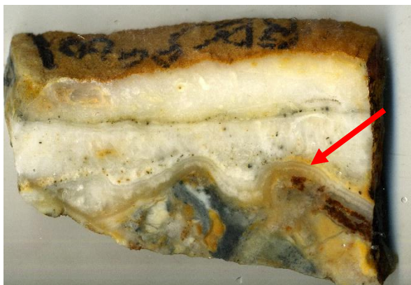
Fig. B-11. Images that indicate overprinting epithermal features. Top left is a sample of quartz vein from Berlin Canyon that contains banded, colloform vein textures (indicated by red arrow). Bottom is an image of bladed quartz and calcite, which indicates boiling conditions. Found in the Grantsville pit.
