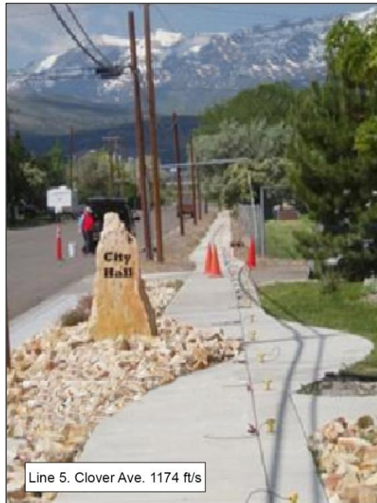
Figure 20. Seismometer array down the sidewalk in front of the City Hall. Photograph by C.M. dePolo.
