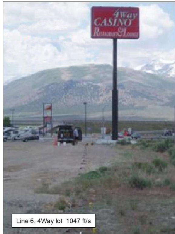
Figure 26. Seismic array used for Line 6 in the 4-Way parking lot.
